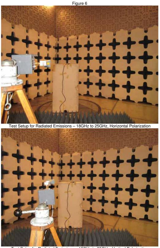
Test Setup for Radiated Emissions – 18GHz to 25GHz, Vertical Polarization
