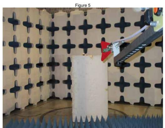
Test Setup for Radiated Emissions – 1GHz to 18GHz, Horizontal Polarization
