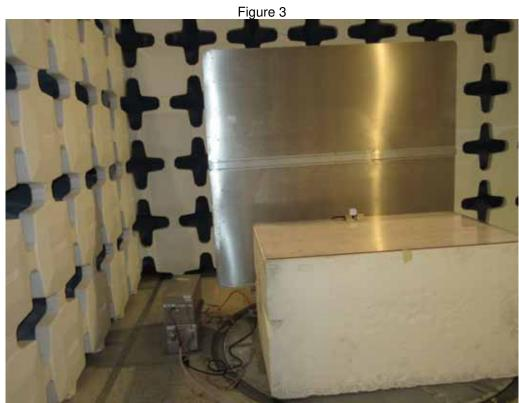
Test Setup for Conducted Emissions
