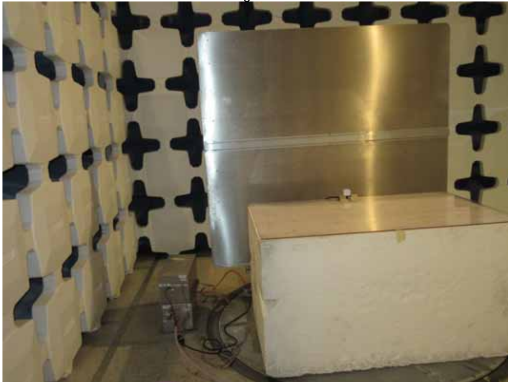
Test Setup for Conducted Emissions
