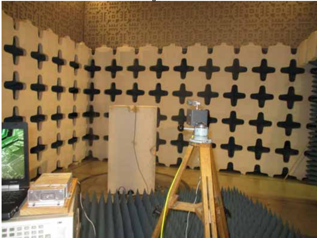
Test Setup for Radiated Emissions – 2GHz to 18GHz, Horizontal Polarization
