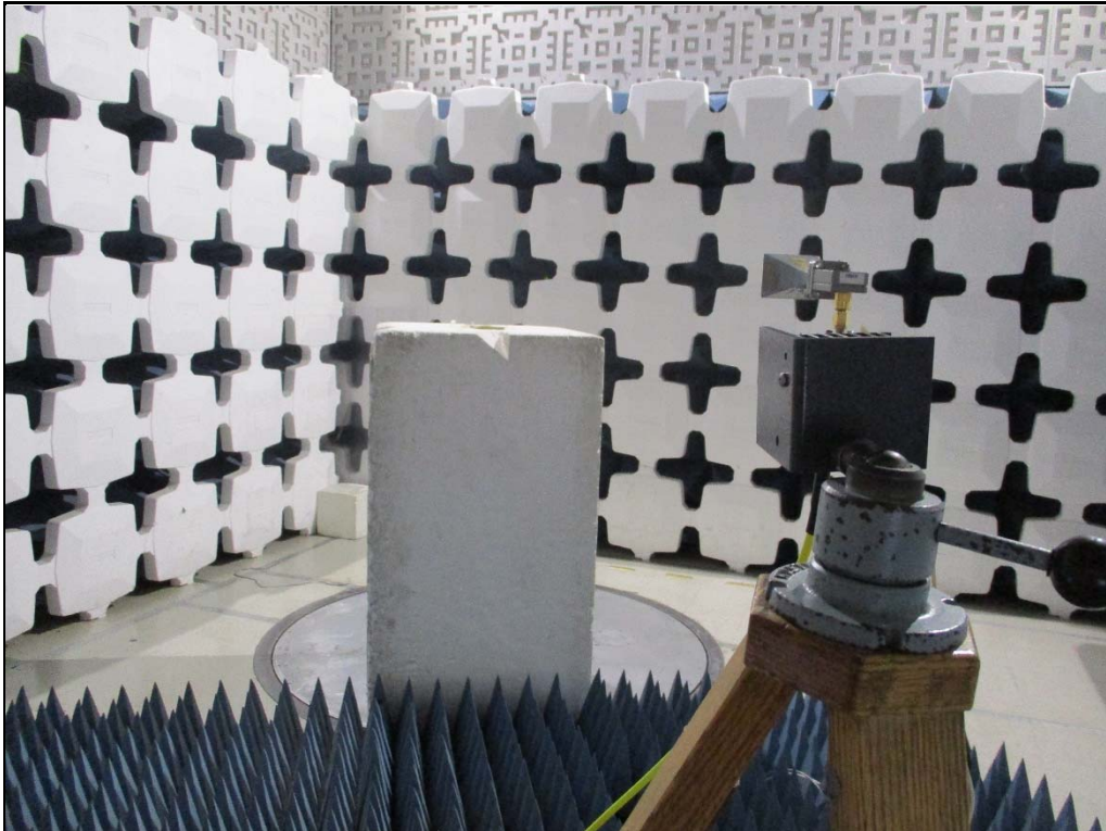
Test Setup for Spurious Radiated Emissions, 18GHz to 25GHz – Antenna Polarization Vertical
