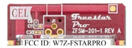
The Freestar Pro module includes an integrated Printed Circuit Board (PCB) trace antenna. An optional MMCX connector can be spedified, providing connection to a 50-ohm external antenna or test equipment.
