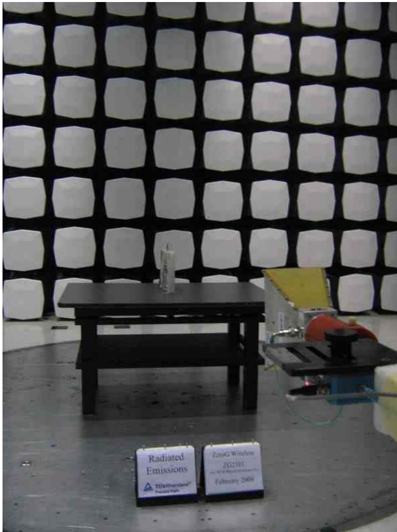
Figure 120: Photo of Test Setup for ZG2101 with 2dBi PCB Antenna #3, 1GHz to 18GHz
