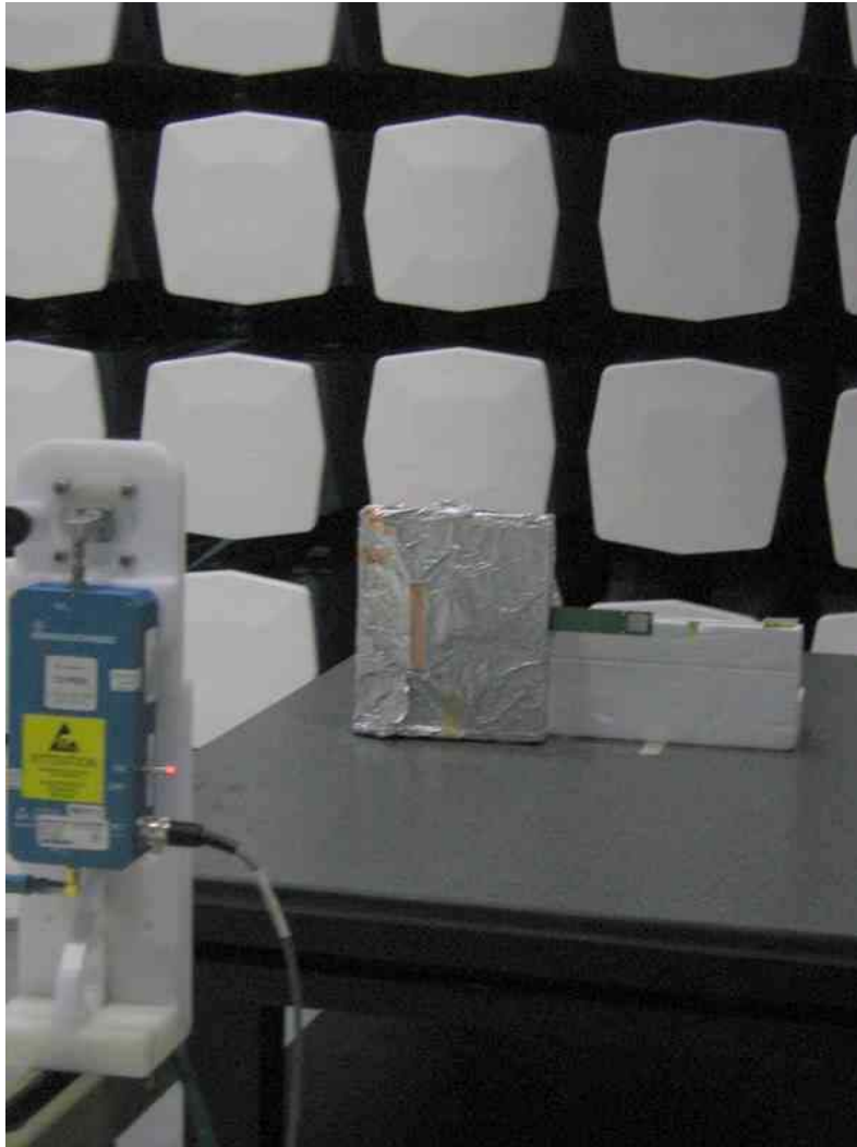
Figure 121: Photo of Test Setup for ZG2101 with 2dBi PCB Antenna #3, 18 GHz to 25GHz
