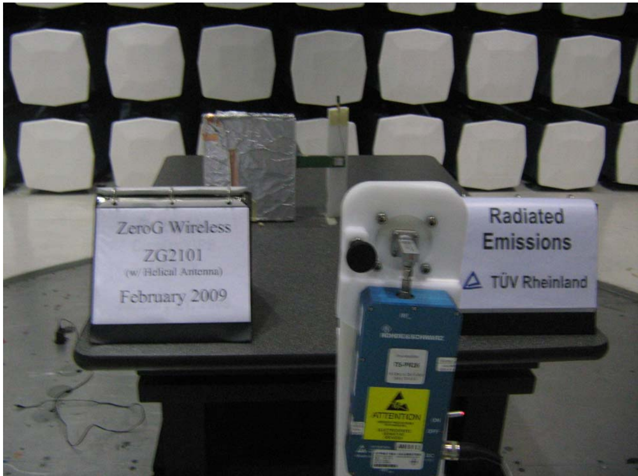
Figure 130: Photo of Test Setup for ZG2101 with Helical Antenna, 18 GHz to 25GHz
