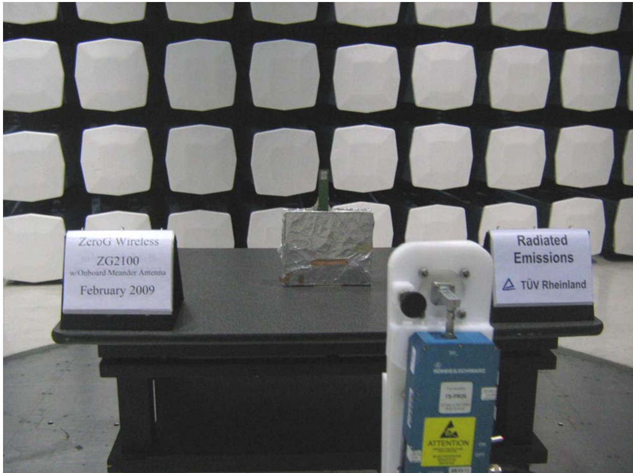
Figure 118: Photo of Test Setup for ZG2100 with On-board PCB Antenna, 18 GHz to 25GHz
