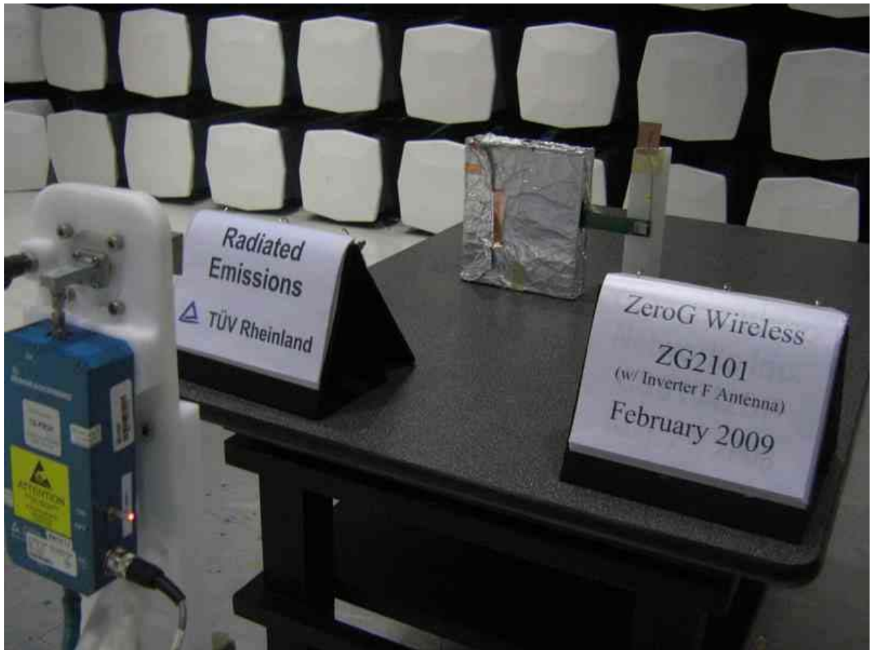
Figure 124: Photo of Test Setup for ZG2101 with Inverter F Antenna, 18 GHz to 25GHz
