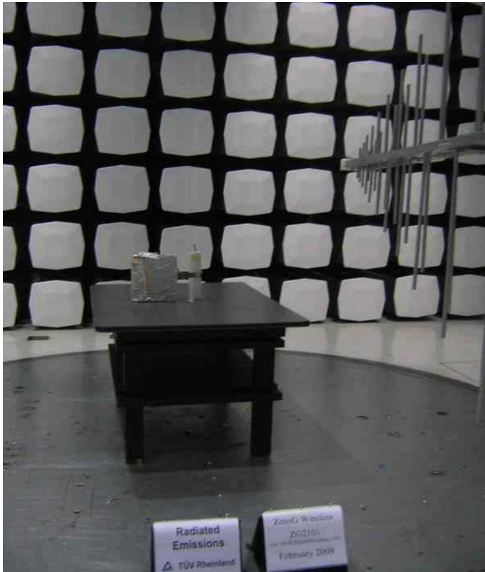
Figure 119: Photo of Test Setup for ZG2101 with 2dBi PCB Antenna #3, 30 to 1000 MHz
