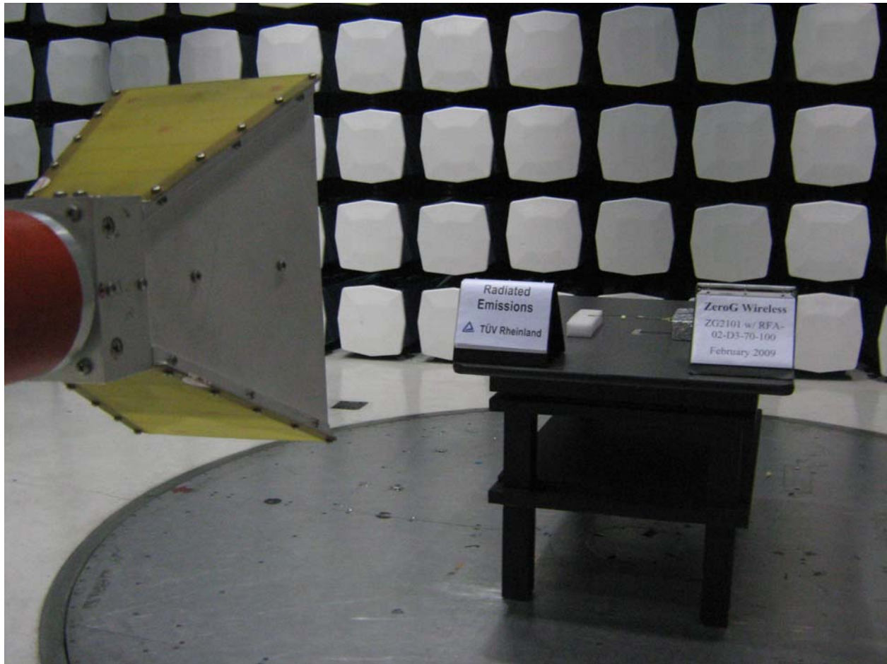
Figure 126: Photo of Test Setup for ZG2101 with RFA-02-D3-70-100 Antenna, 1GHz to 18GHz
