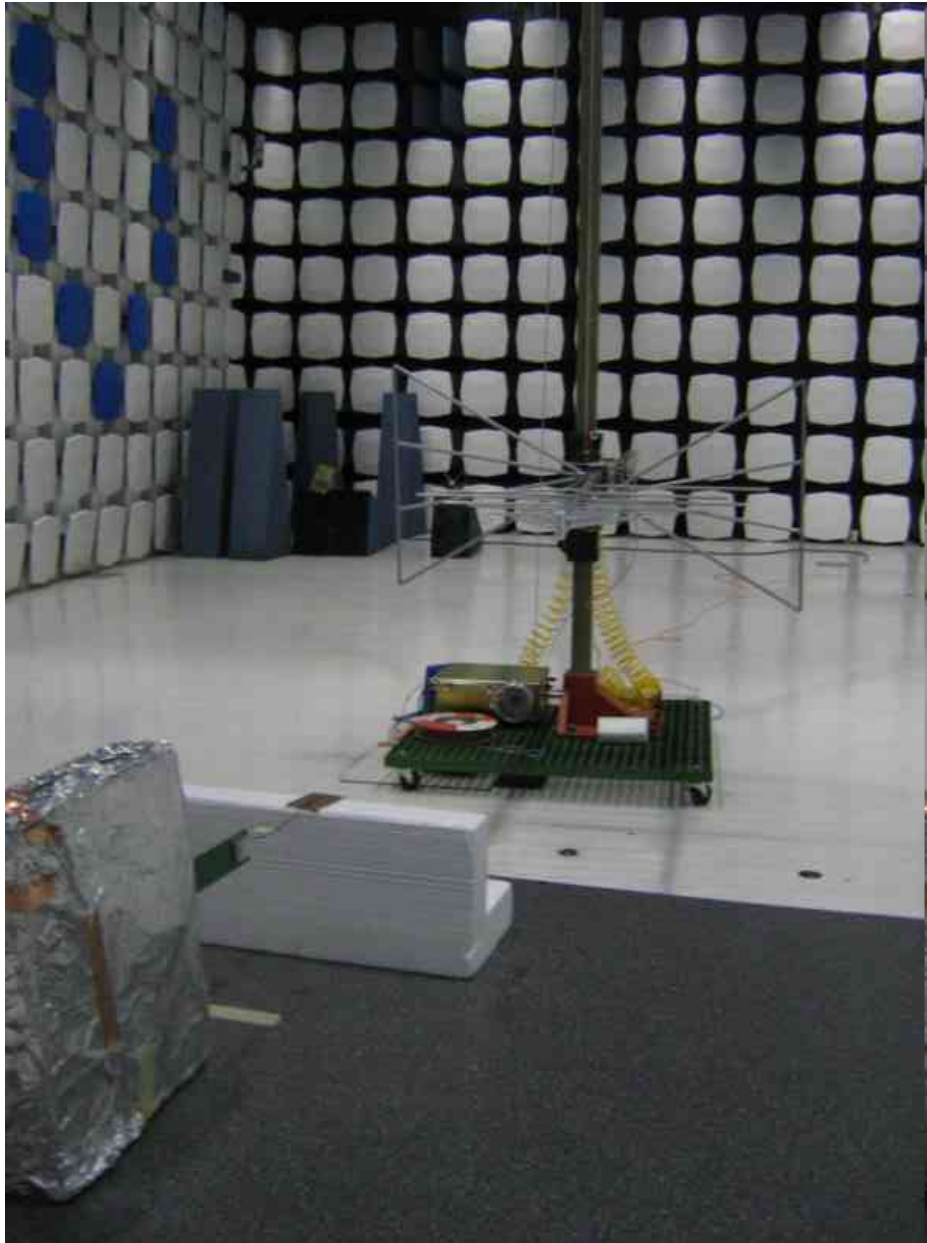
Figure 122: Photo of Test Setup for ZG2101 with Inverter F Antenna, 30 to 1000 MHz
