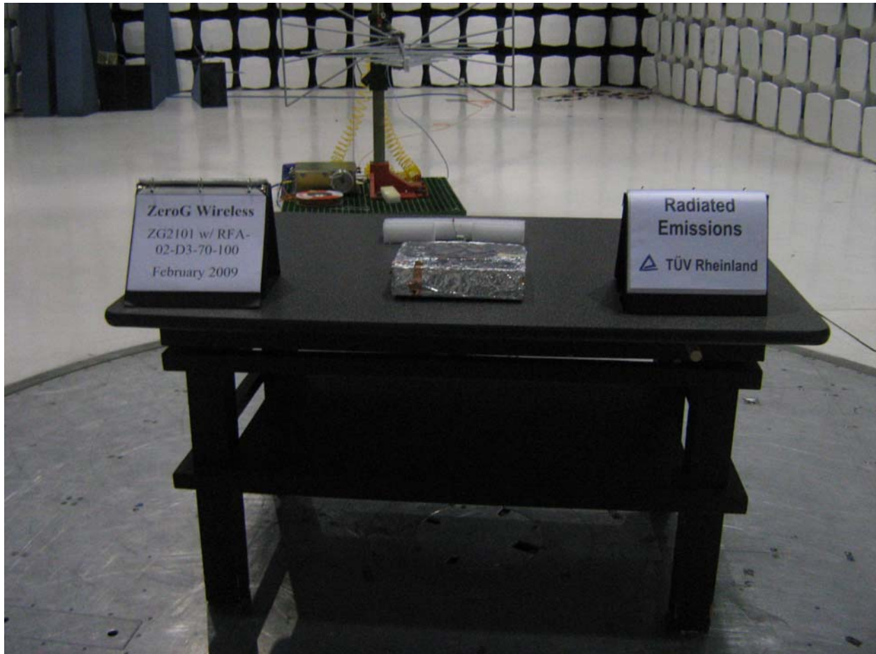
Figure 125: Photo of Test Setup for ZG2101 with RFA-02-D3-70-100 Antenna, 30 to 1000 MHz
