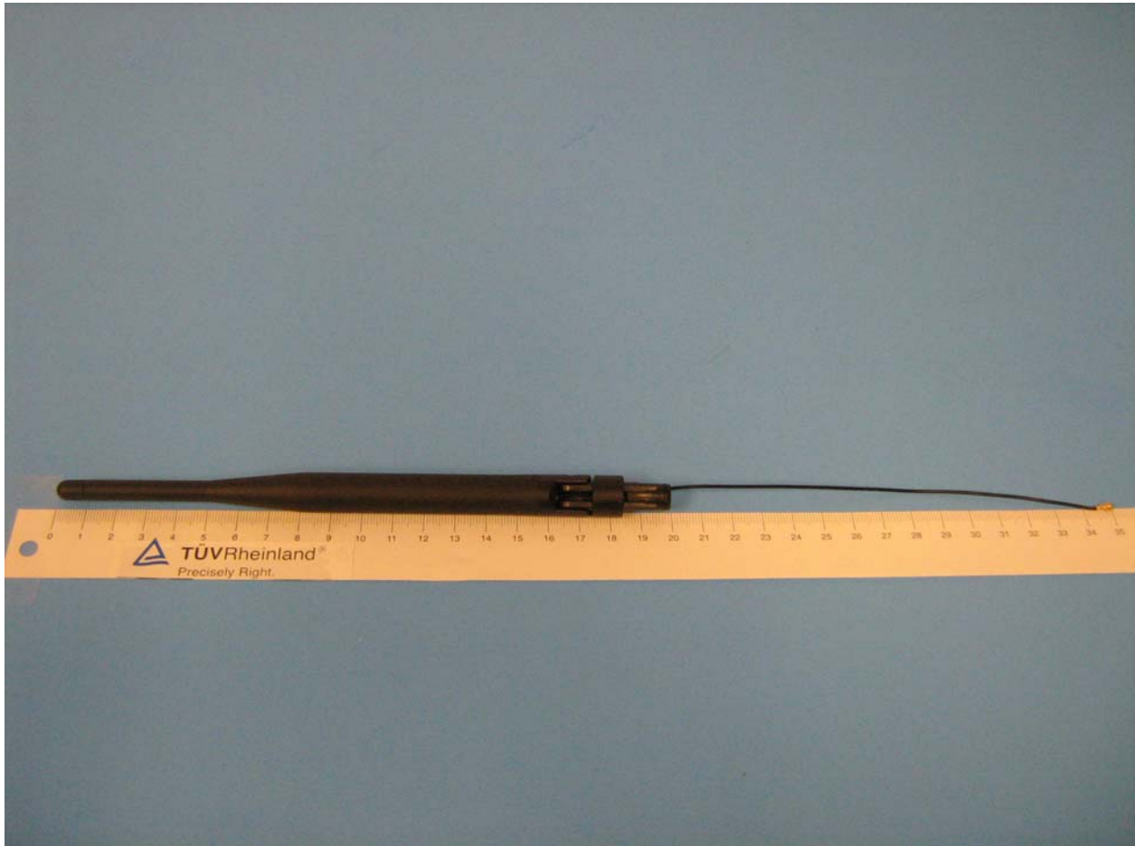
Figure 145: External Antenna for ZG2101 Module – 5dBi Dipole Antenna (WF2400-15001A)
