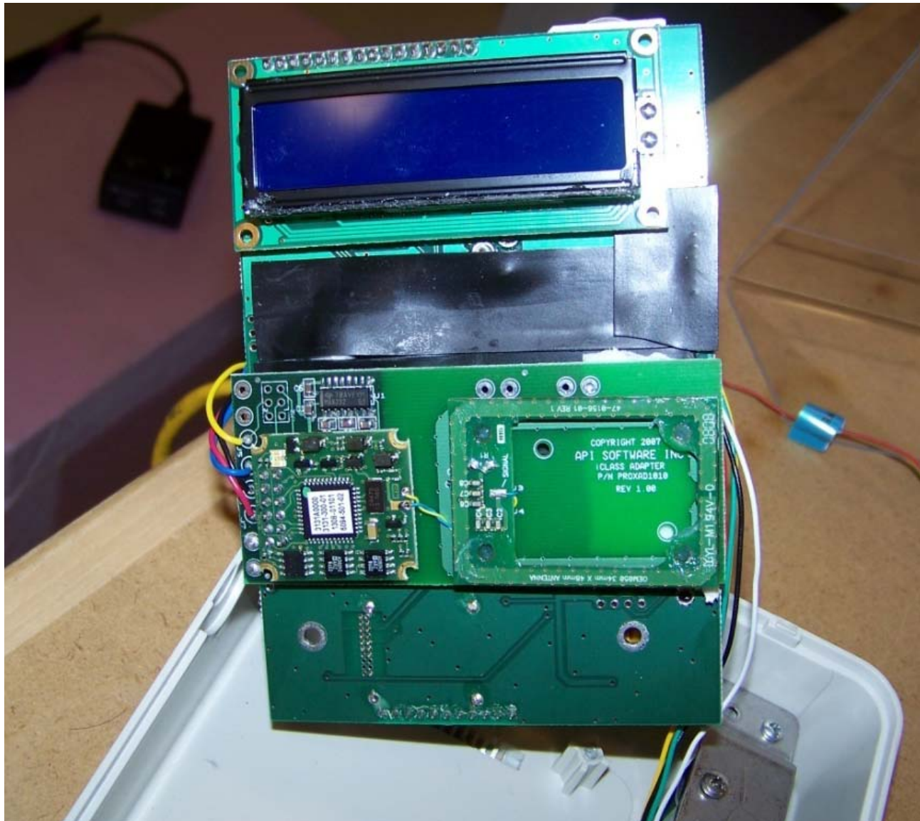
Figure 6: EUT Module Embedded Inside the Host Keypad and Card Reader (Opened for Photo)
