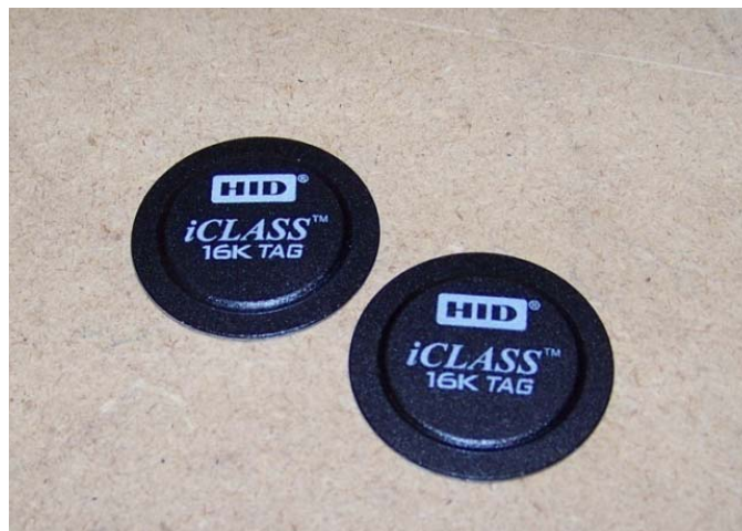
Figure 8: RF ID Tags Used to Verify Operation Of The Host Units
