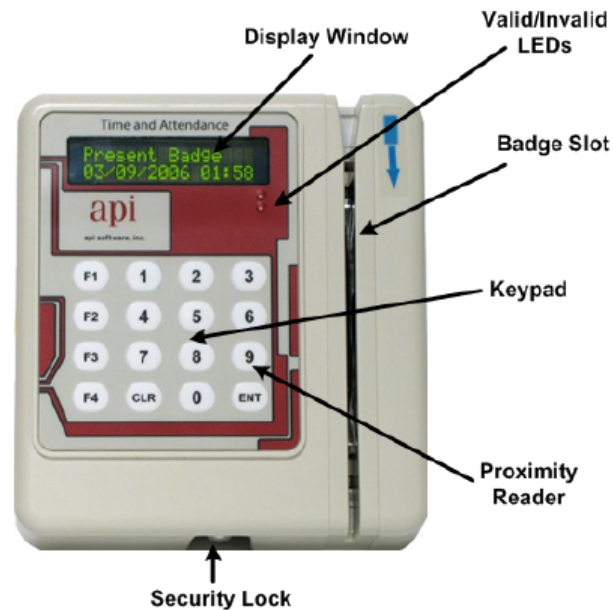
Figure 2: The API Healthcare Module AP500 Badge Reader Used as a Host Controller During Testing
