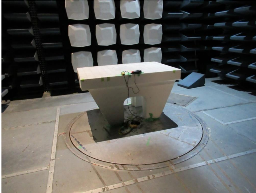
Radiated Emissions performed at the 3m SAC (charging and Battery modes)
