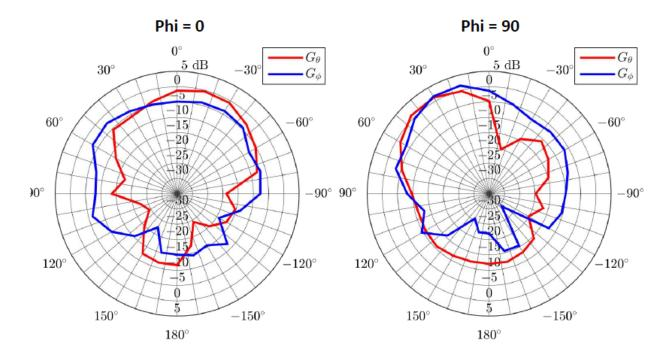
Cellular Linear Gain vs Phi Angle 1.85 GHz
