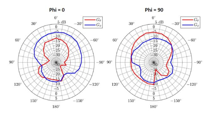
Cellular Linear Gain vs Phi Angle 0.75 GHz
