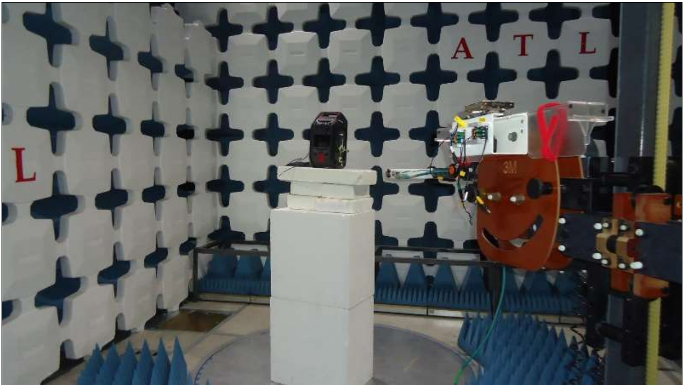
Radiated Emission Test Setup - Front View
