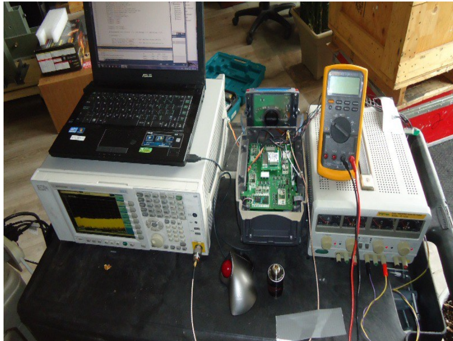
Figure 4.14 – RF Conducted Tests Test Setup
