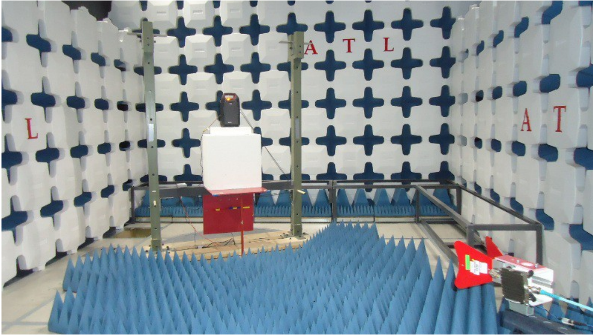
Figure 4.8 - Radiated Emission Test Setup - Front View
