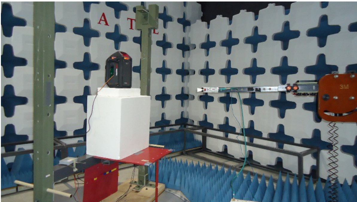
Figure 4.11 - Radiated Emission Test Setup - Side View
