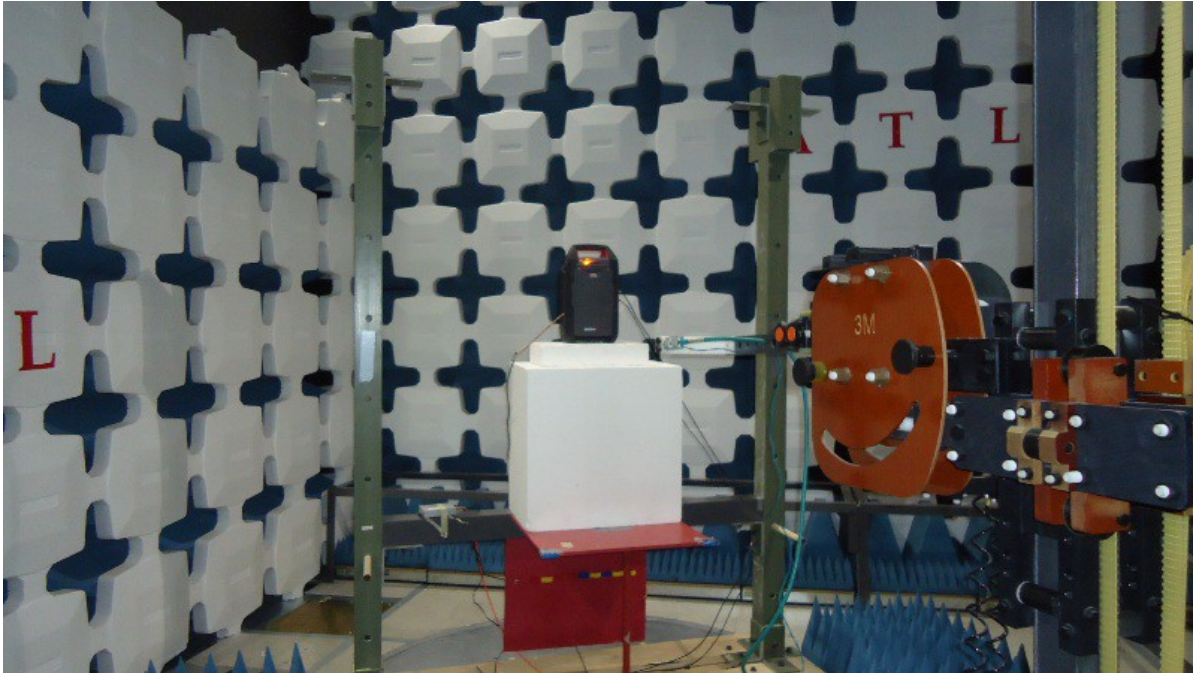
Figure 4.10 - Radiated Emission Test Setup - Front View
