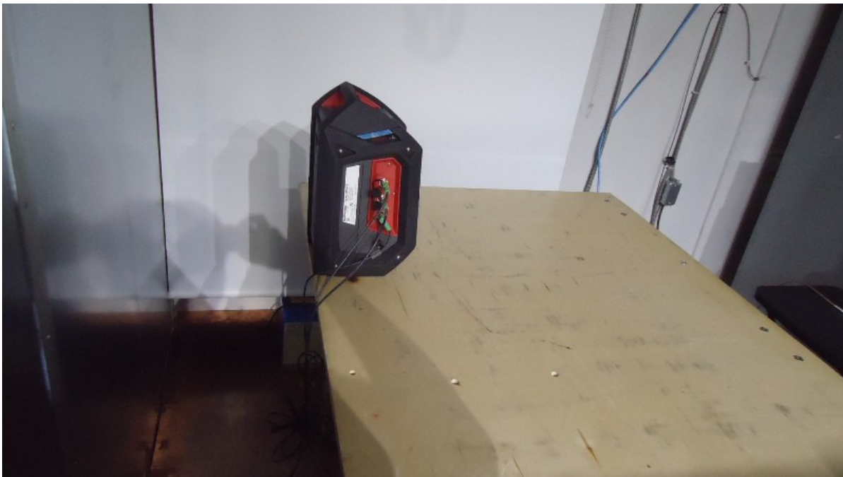
Figure 4.13 - Conducted Emission Test Setup - Side View
