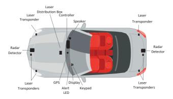
The Controller is the brain of the R9 system. It provides power to and communications between the elements that attach to it.
