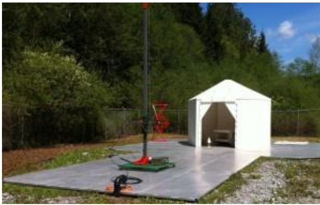
10 m Open Area Test Site (OATS) in British Columbia, Canada
