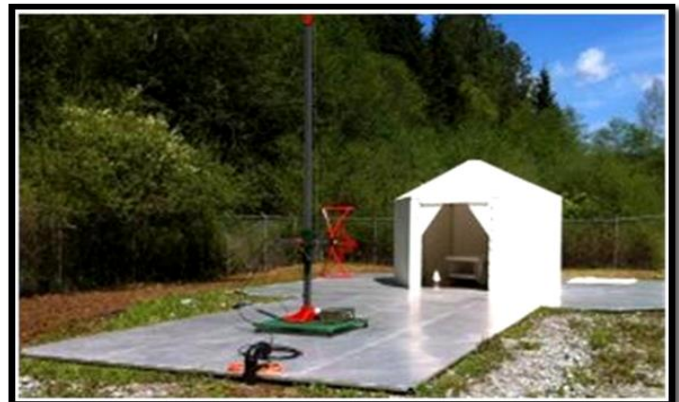
10m Open Area Test Site (OATS) Malcom Knapp Research Forest, Maple Ridge, BC
