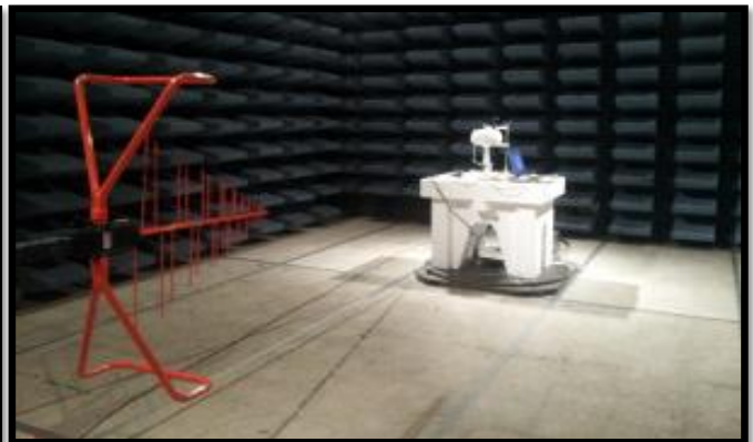
3m Semi-Anechoic Chamber (SAC) Burnaby, BC
