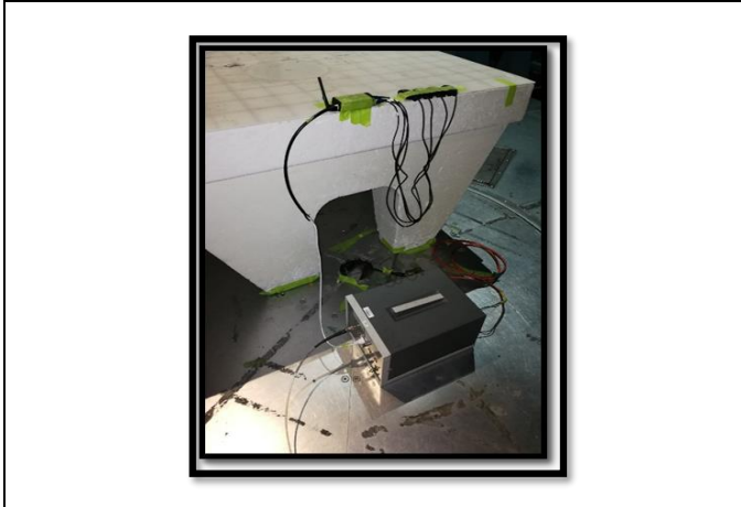
Figure R3: Conducted Emissions Test Setup
