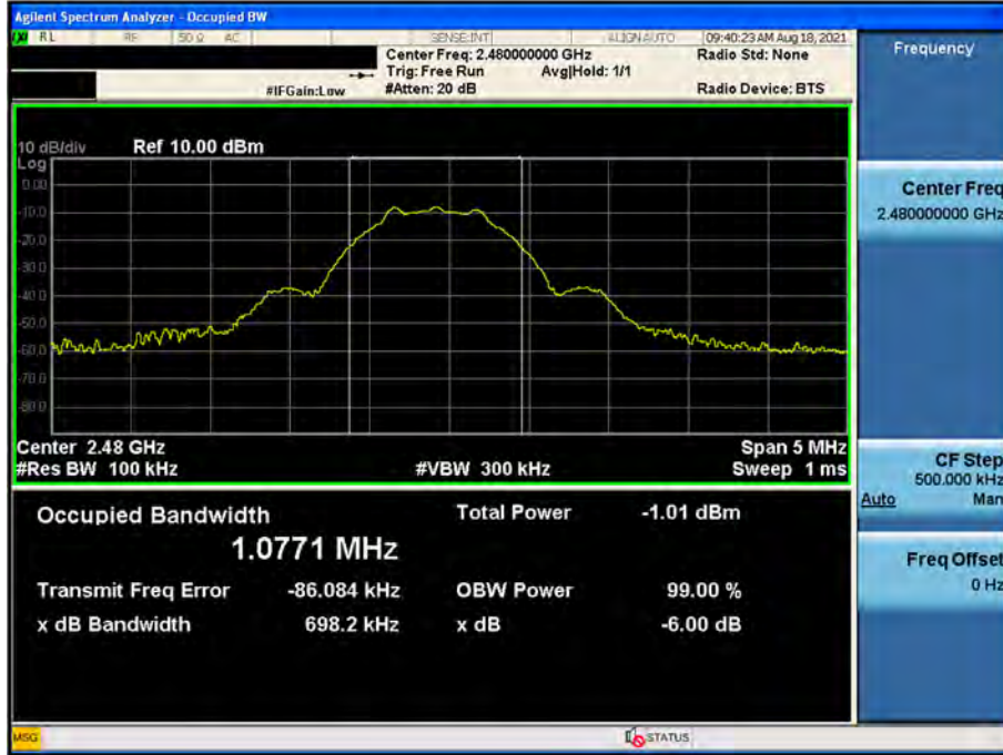
6 dB Bandwidth plot (High-CH 39)
