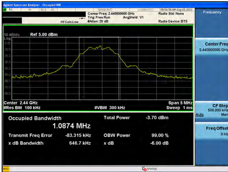
6 dB Bandwidth plot (Mid-CH 19)
