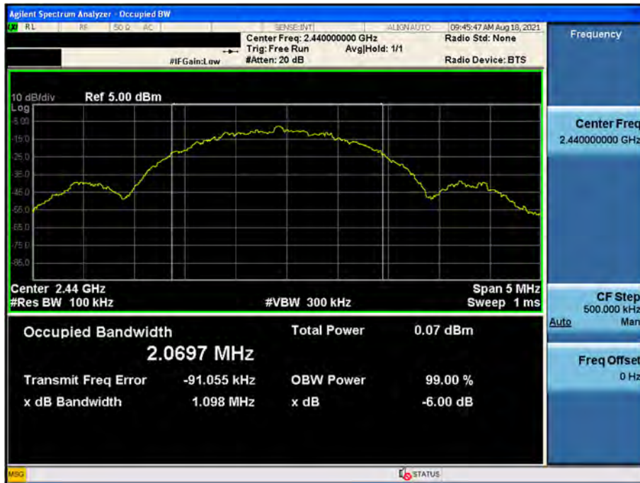
6 dB Bandwidth plot (Mid-CH 19)
