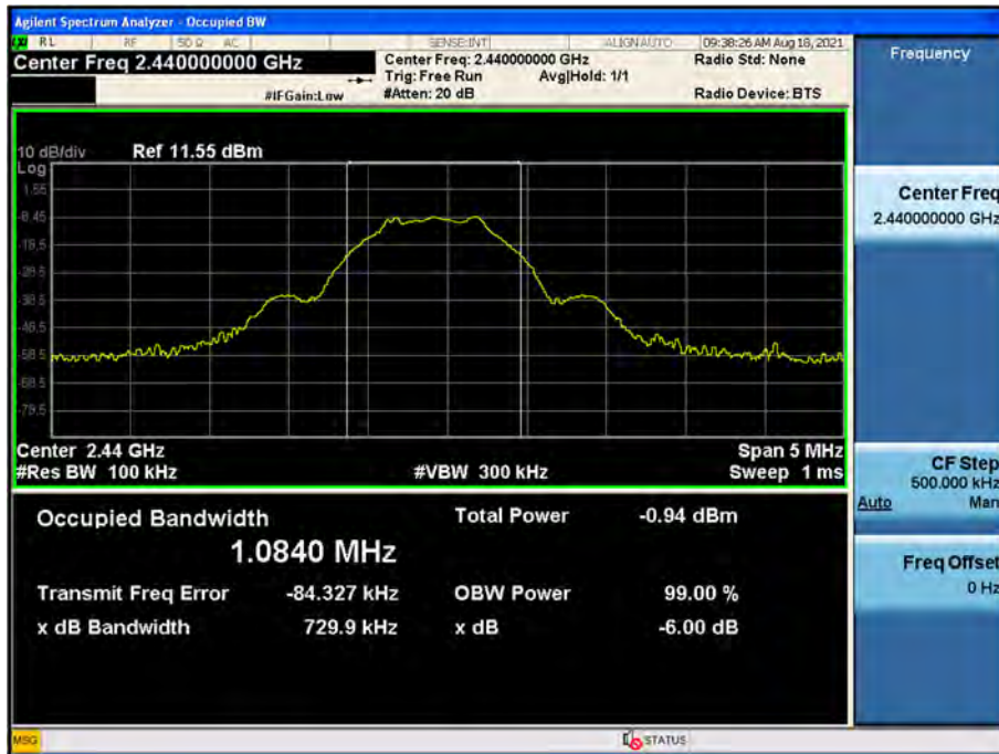
6 dB Bandwidth plot (Mid-CH 19)
