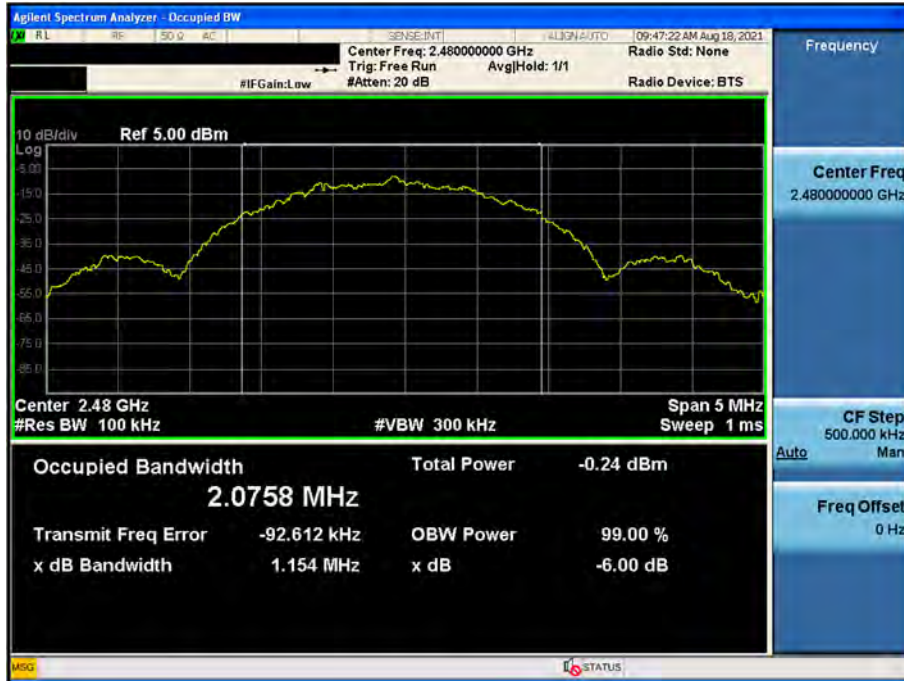
6 dB Bandwidth plot (High-CH 39)
