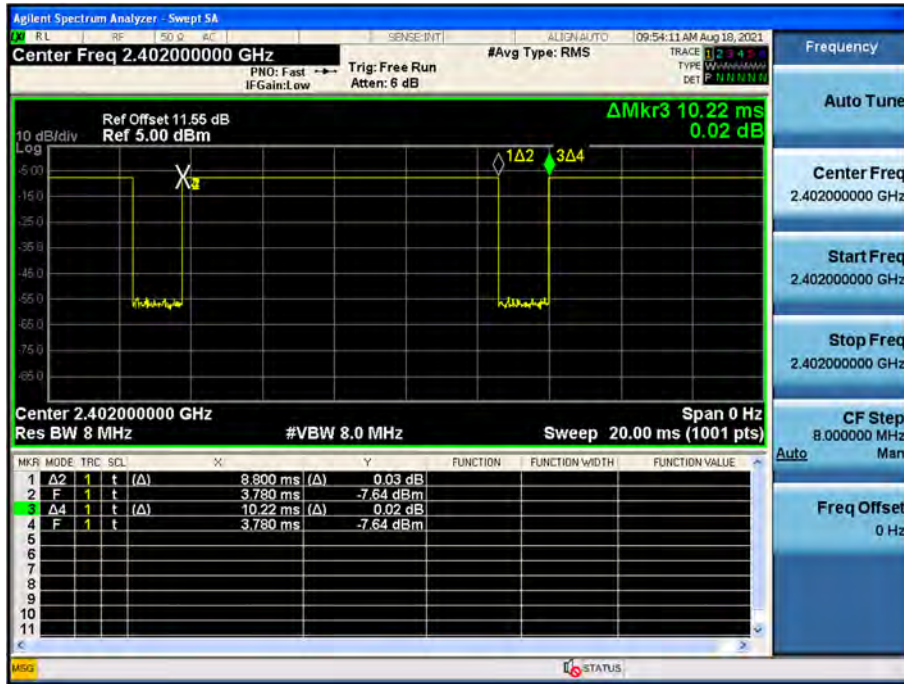
Duty Cycle (Low-CH 0)
