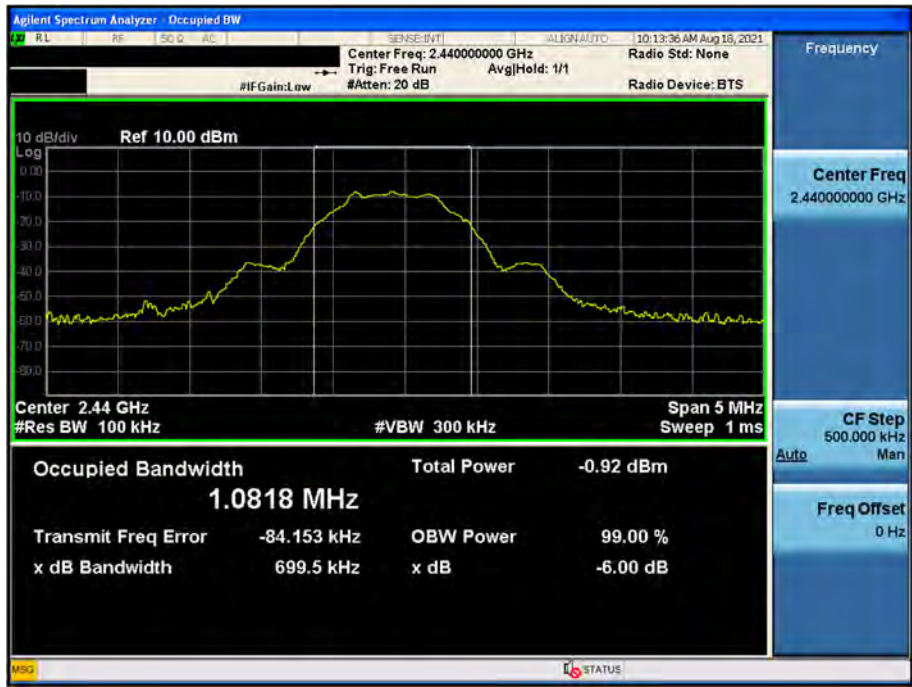
6 dB Bandwidth plot (Mid-CH 19)
