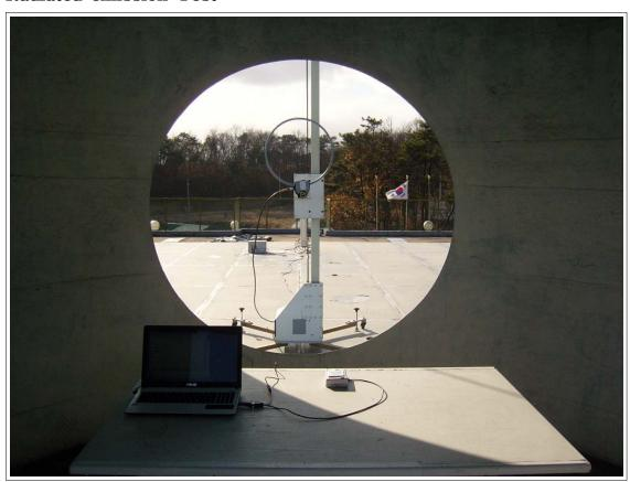
Radiated emission Test
