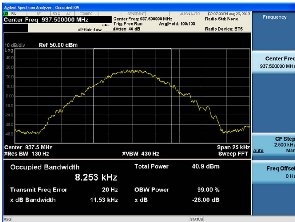
3 dB above the AGC threshold output / 900I_PA(935 ~ 940 MHz) / Downlink
