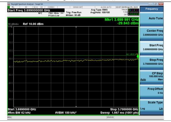
+3 dB above Out-of-band (single test signal) / 3.7 GHz Service (Ant1) / Downlink / 5G NR 60 MHz / Lower
