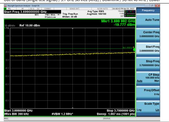
Out-of-band (single test signal) / 3.7 GHz Service (Ant2) / Downlink / 5G NR 40 MHz / Lower
