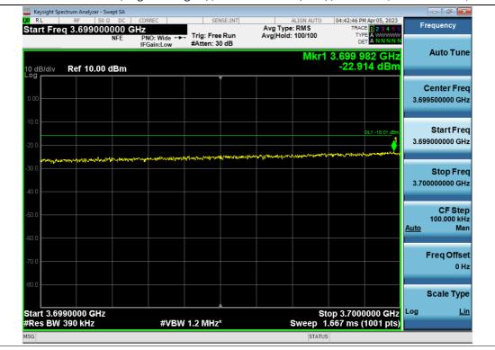
+3 dB above Out-of-band (single test signal) / 3.7 GHz Service (Ant1) / Downlink / 5G NR 40 MHz / Lower
