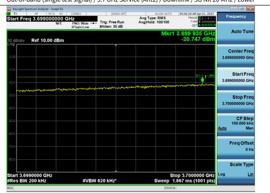
Out-of-band (single test signal) / 3.7 GHz Service (Ant2) / Downlink / 5G NR 20 MHz / Lower
