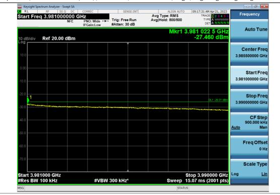
Spurious / 3.7 GHz Service (Ant2) / Downlink / 5G NR 20 MHz / High / High Edge ~ High Edge + 10 MHz
