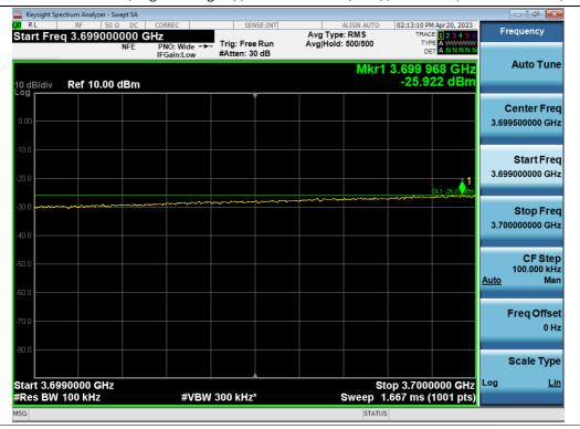
+3 dB above Out-of-band (single test signal) / 3.7 GHz Service (Ant2) / Downlink / 5G NR 100 MHz / Lower
