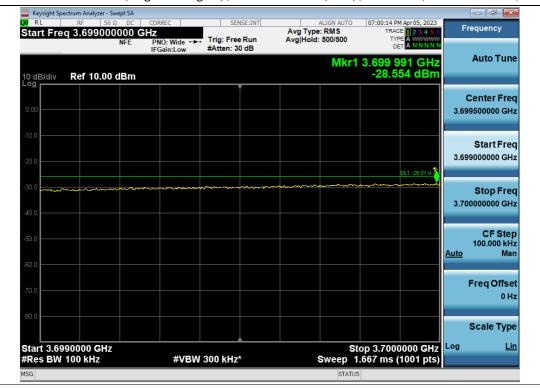
+3 dB above Out-of-band (single test signal) / 3.7 GHz Service (Ant1) / Downlink / 5G NR 100 MHz / Lower
