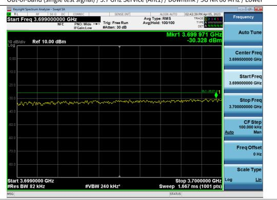
Out-of-band (single test signal) / 3.7 GHz Service (Ant1) / Downlink / 5G NR 80 MHz / Lower
