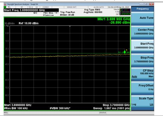
Out-of-band (single test signal) / 3.7 GHz Service (Ant2) / Downlink / 5G NR 100 MHz / Lower
