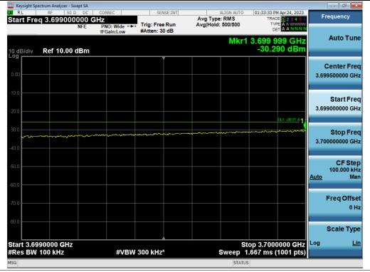
+3 dB above Out-of-band (single test signal) / 3.7 GHz Service (Ant1) / Downlink / 5G NR 4 Carriers(100 + 60 + 80 + 40) / Upper
