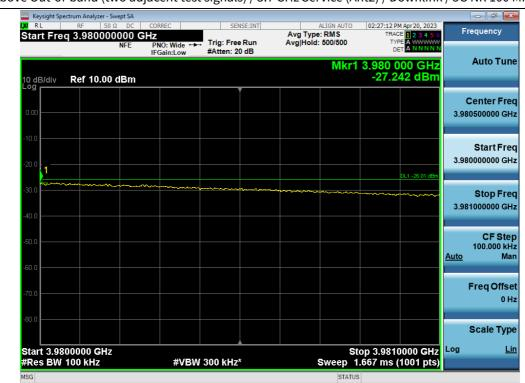
+3 dB above Out-of-band (two adjacent test signals) / 3.7 GHz Service (Ant2) / Downlink / 5G NR 100 MHz / Upper
