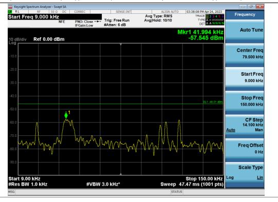
Spurious / 3.7 GHz Service (Ant2) / Downlink / 5G NR 4 Carriers(100 + 60 + 80 + 40) / Middle / 9 kHz ~ 150 kHz
