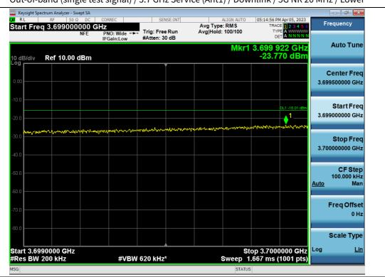
Out-of-band (single test signal) / 3.7 GHz Service (Ant1) / Downlink / 5G NR 20 MHz / Lower
