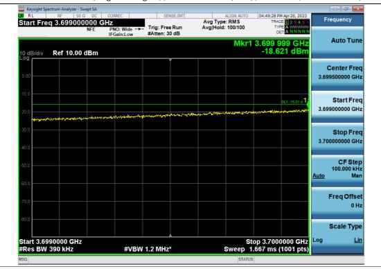
+3 dB above Out-of-band (single test signal) / 3.7 GHz Service (Ant2) / Downlink / 5G NR 40 MHz / Lower
