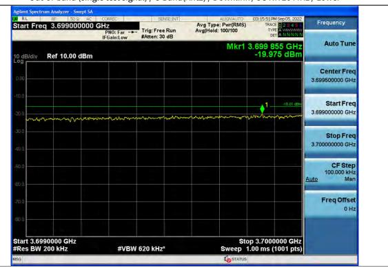
Out-of-band (single test signal) / C-Band(Ant2) / Downlink / 5G NR 20 MHz / Lower
