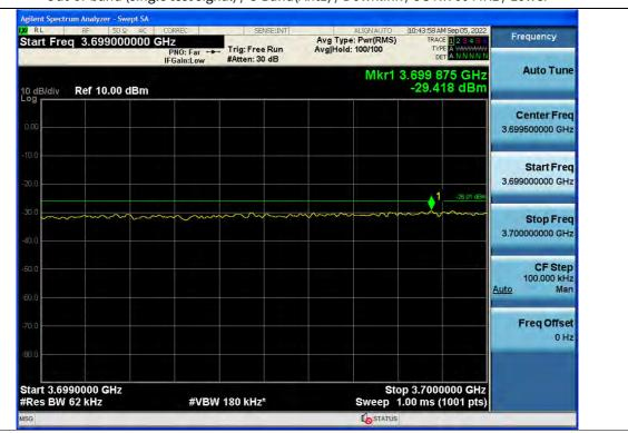
Out-of-band (single test signal) / C-Band(Ant1) / Downlink / 5G NR 60 MHz / Lower
