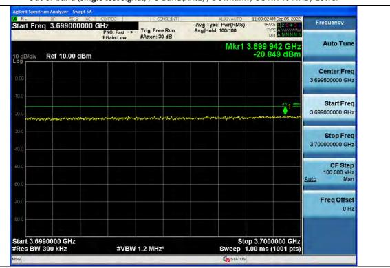
Out-of-band (single test signal) / C-Band(Ant1) / Downlink / 5G NR 40 MHz / Lower
