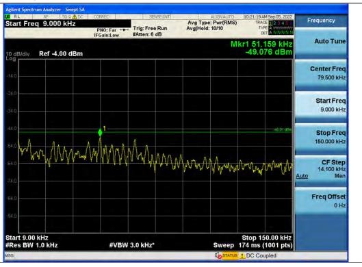
Spurious / C-Band(Ant1) / Downlink / 5G NR 80 MHz / Middle / 9 kHz ~ 150 kHz
