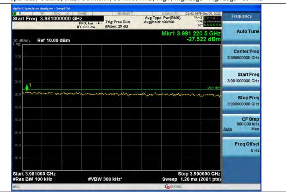
Spurious / C-Band(Ant2) / Downlink / 5G NR 60 MHz / High / High Edge ~ High Edge + 10 MHz
