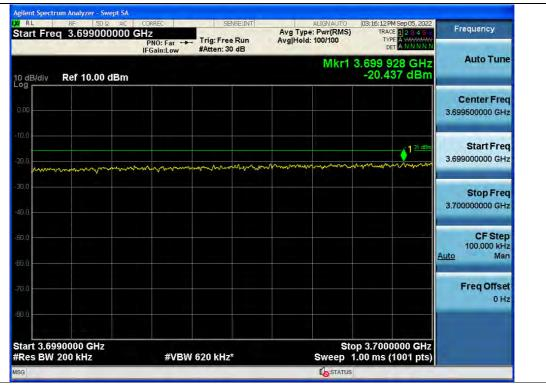
+3 dB above Out-of-band (single test signal) / C-Band(Ant2) / Downlink / 5G NR 20 MHz / Upper
