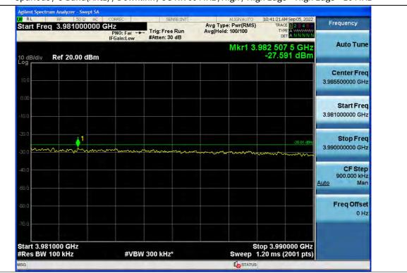
Spurious / C-Band(Ant1) / Downlink / 5G NR 60 MHz /High / High Edge ~ High Edge + 10 MHz
