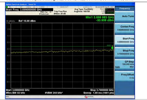
Out-of-band (two adjacent test signals) / C-Band(Ant2) / Downlink / 5G NR 80 MHz / Lower
