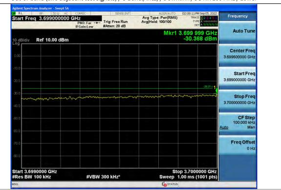
Out-of-band (two adjacent test signals) / C-Band(Ant2) / Downlink / 5G NR 100 MHz / Lower
