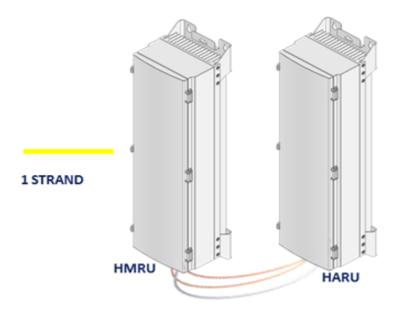
Figure 3. HROU consists of 2 unit
