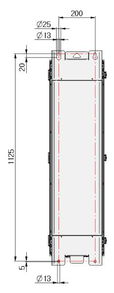
Figure 18. Dimension used to install HROU on the WALL
