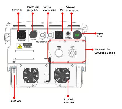
Figure 16. The name of each port on the bottom of HROU
