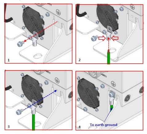
Figure 22. How to install Ground Terminal
