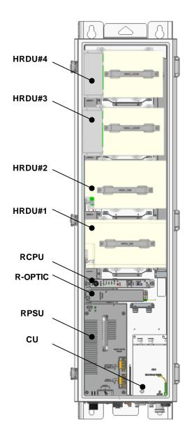
Figure 6. Inside of Remote Unit
