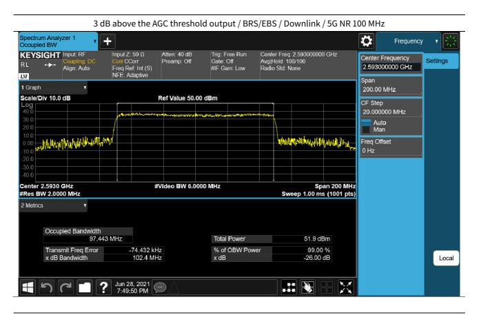
3 dB above the AGC threshold Input / BRS/EBS / Downlink / 5G NR 100 MHz
