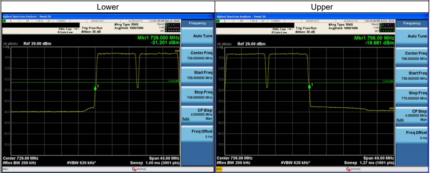
Out-of-band (two adjacent test signals) / 700 LTE / Downlink / LTE 10 MHz
