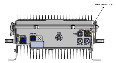
Optical cables should be inserted into Optic Port outside of N2ROU. Through GUI, check if PD value of ROPTIC is in a tolerable range (+5~1dBm).
