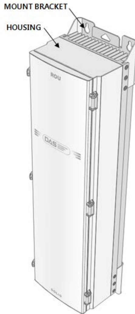
Figure 4.1 – Exterior of Remote Unit
