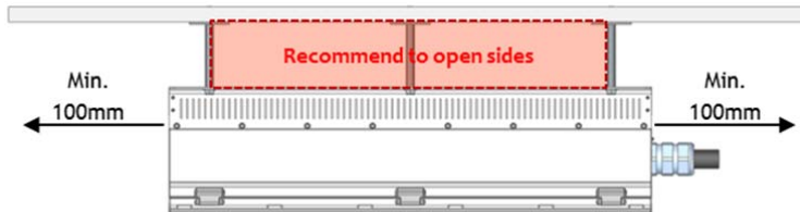
Figure 4.4 – Installation Clearance
