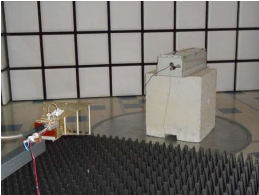
Radiated Test Setup
