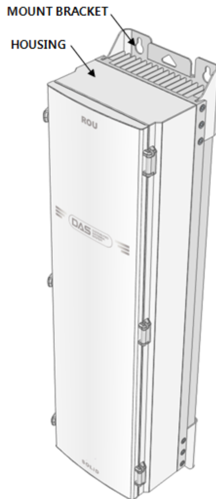
Figure 4.1 – Exterior of Remote Unit
