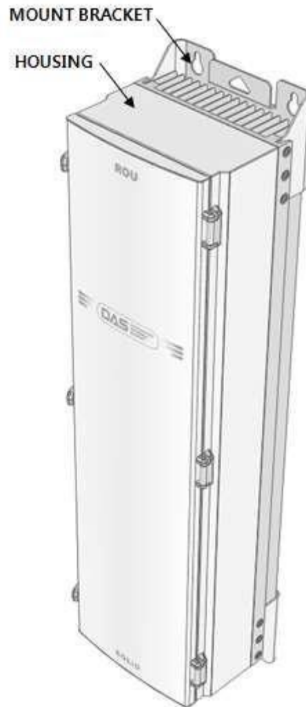
Figure 4.1 – Exterior of Remote Unit
