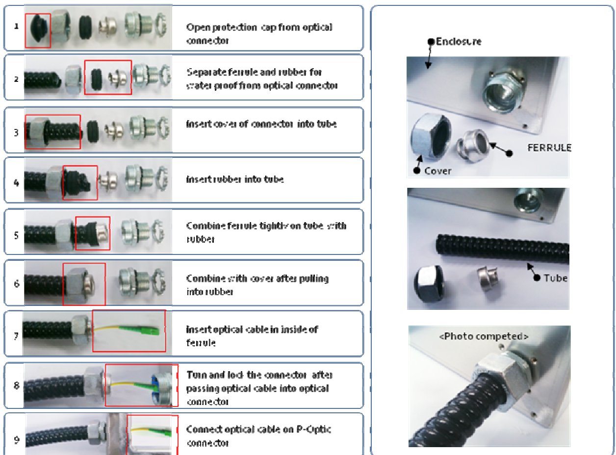
Figure 5.8 – How to work optical port
