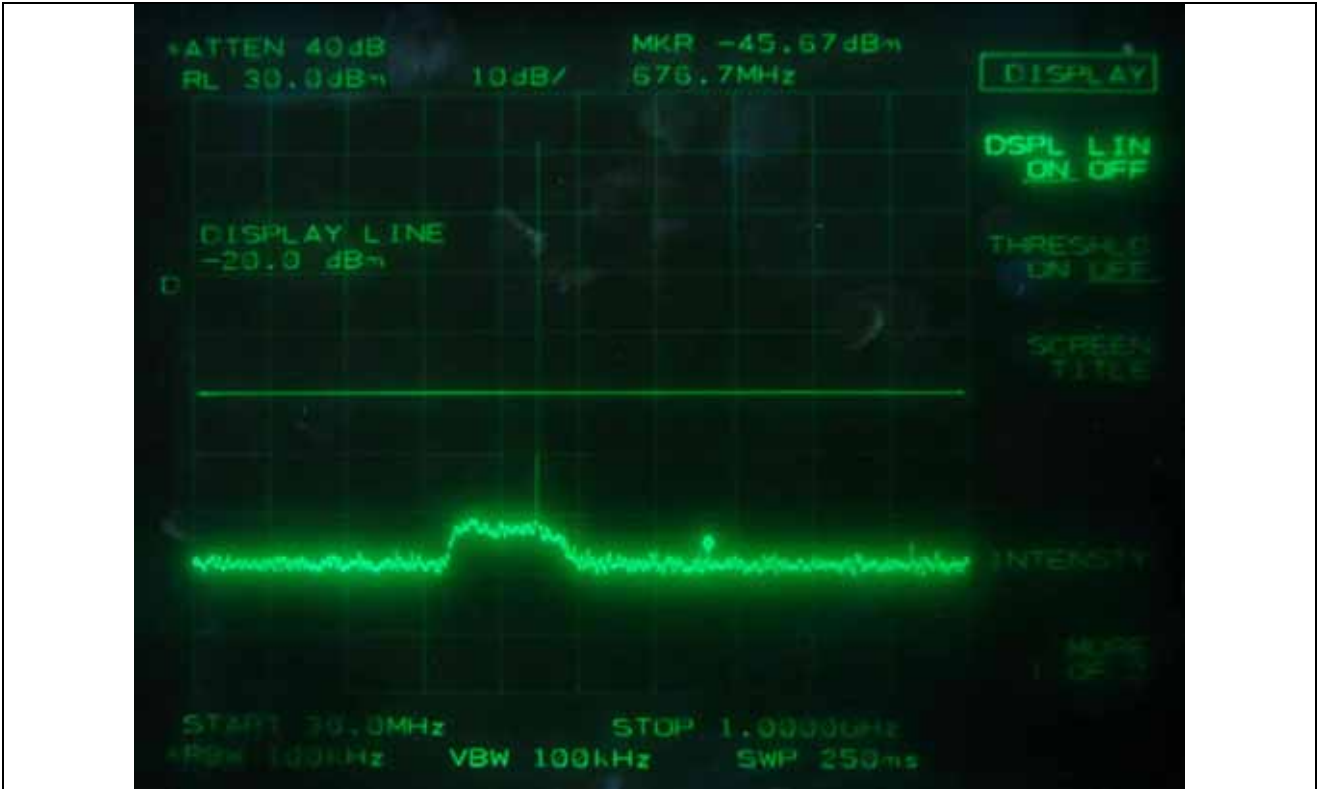
FM with an external 9 600 b/s random data source, Channel Spacing 12.5 kHz - Middle Channel
