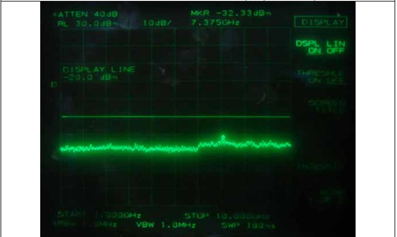
FM with an external 9 600 b/s random data source, Channel Spacing 12.5 kHz - High Channel
