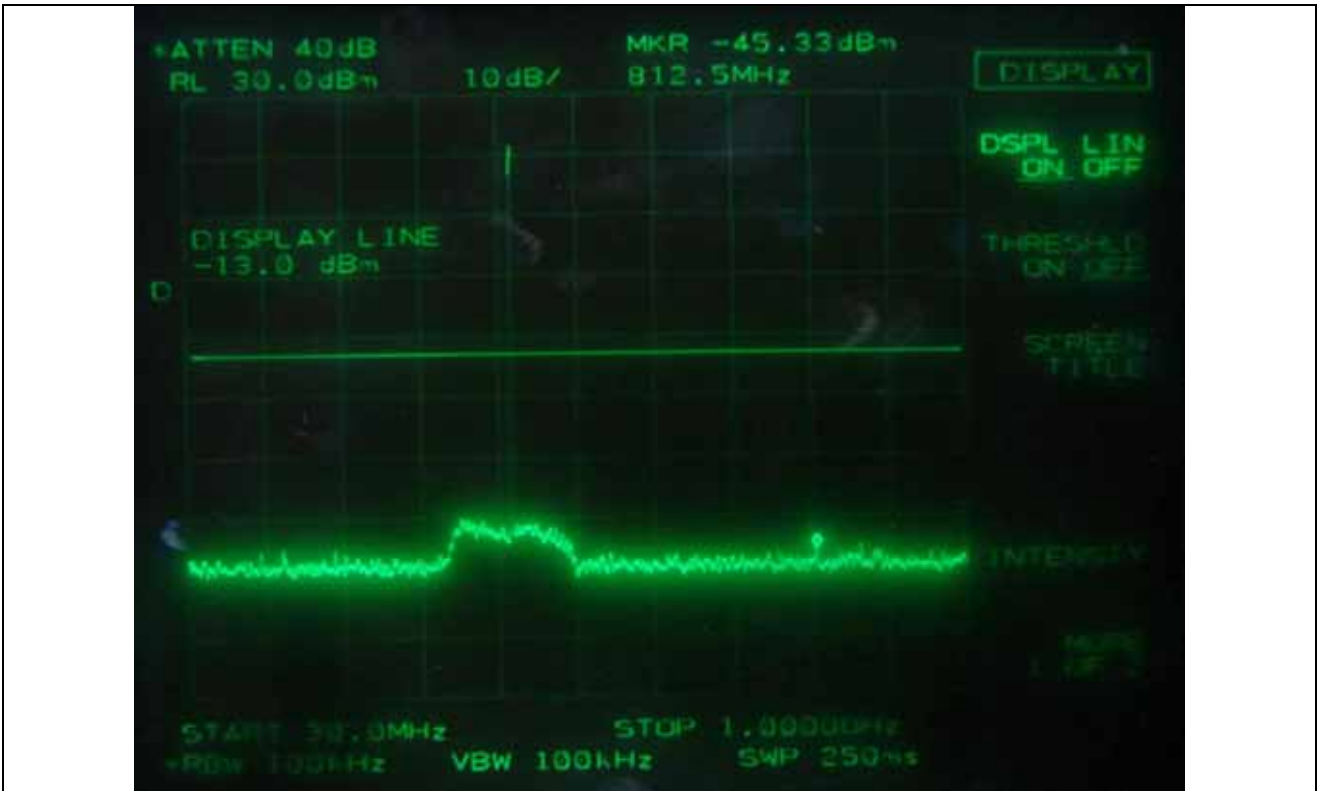
FM with an external 9 600 b/s random data source, Channel Spacing 25 kHz - Low Channel
