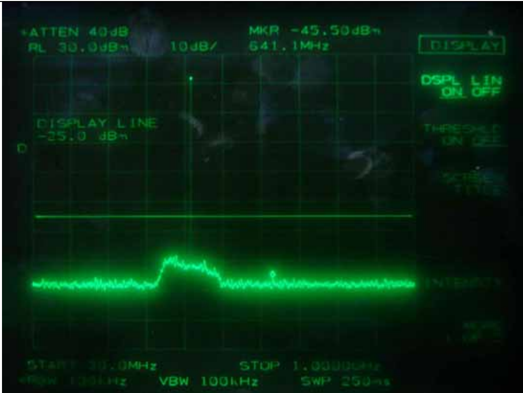
FM with an external 9 600 b/s random data source, Channel Spacing 6.25 kHz - High Channel
