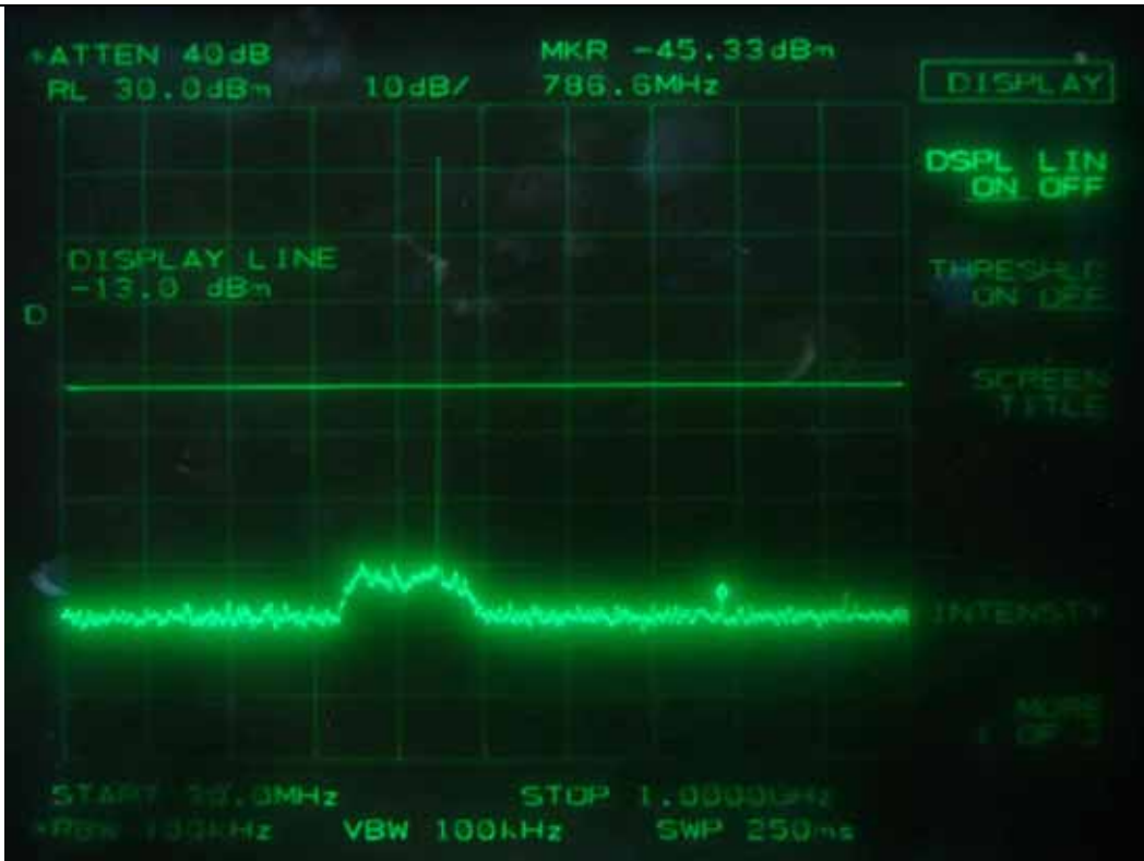
FM with an external 9 600 b/s random data source, Channel Spacing 25 kHz - Middle Channel
