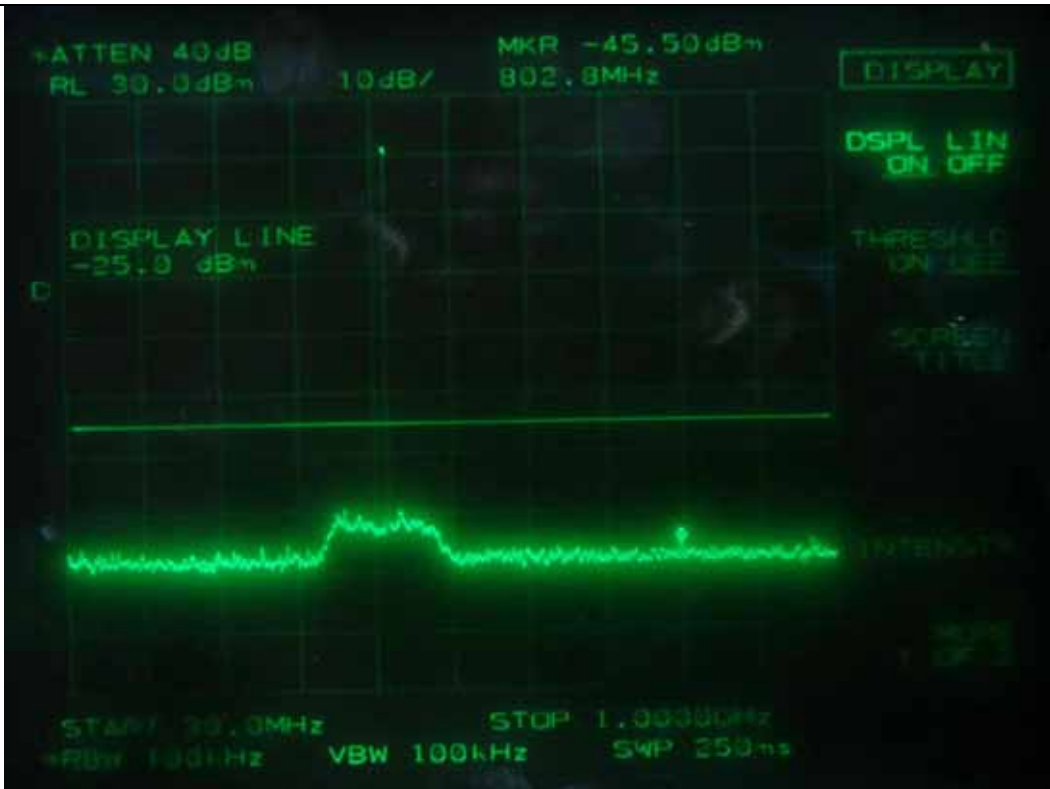
FM with an external 9 600 b/s random data source, Channel Spacing 6.25 kHz - Low Channel
