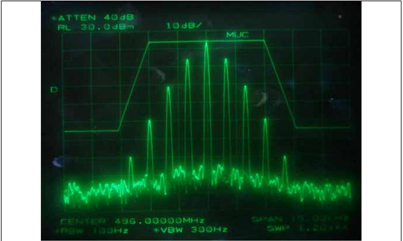
FM with 2.5 kHz sine wave signal, Channel Spacing 6.25 kHz - High Channel
