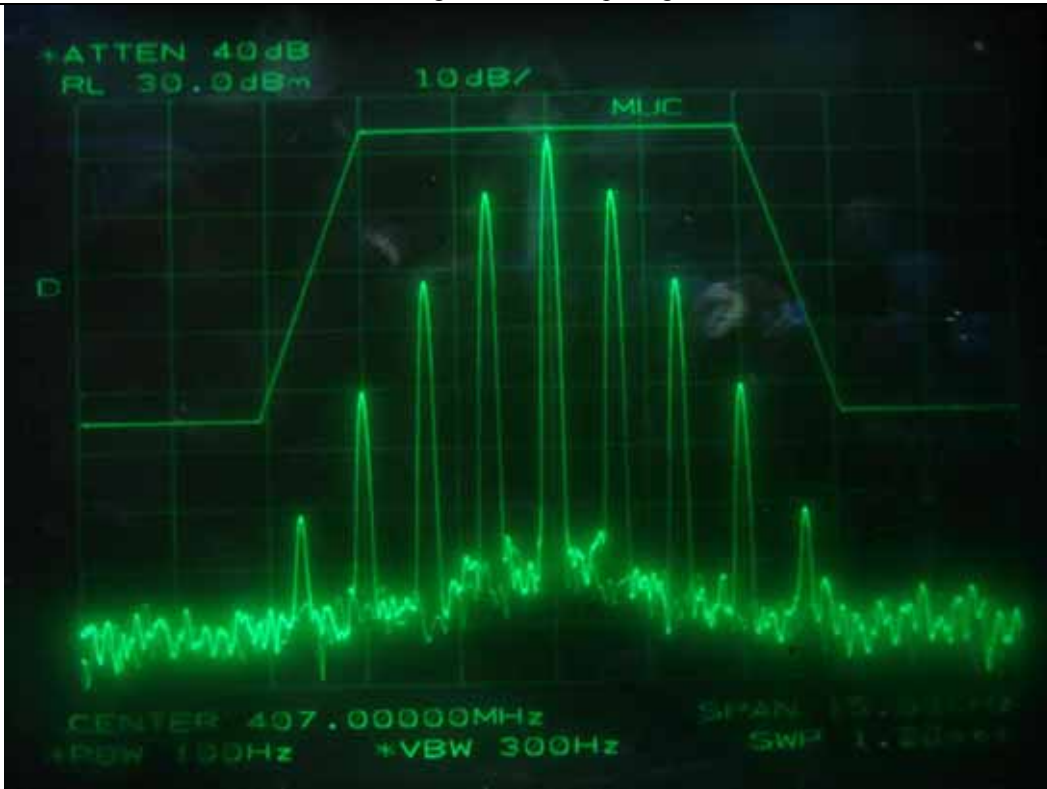
FM with 2.5 kHz sine wave signal, Channel Spacing 6.25 kHz - Middle Channel
