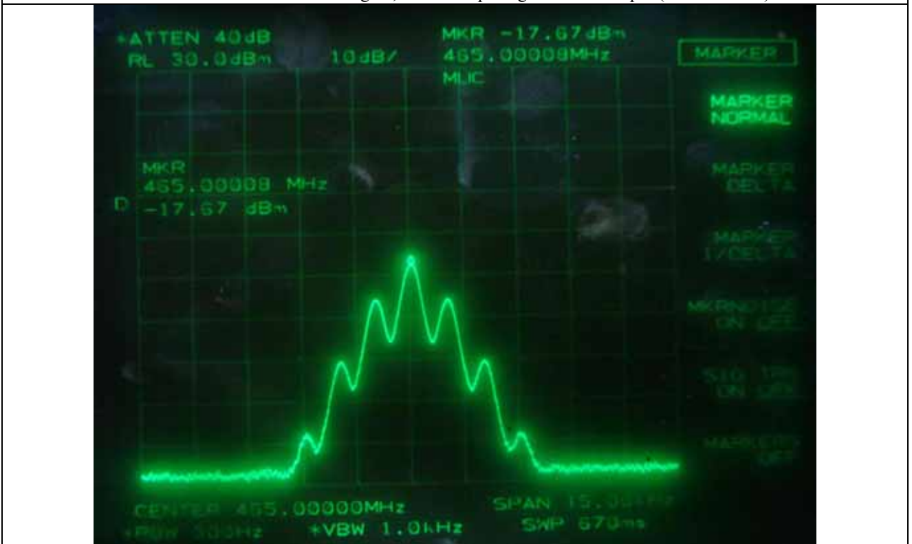
FM with 2.5 kHz sine wave signal, Channel Spacing 6.25 kHz - Input (Middle Channel)
