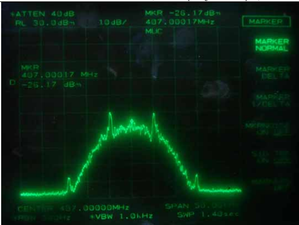
FM with an external 9 600 b/s random data source, Channel Spacing 25 kHz - Input (Middle Channel)
