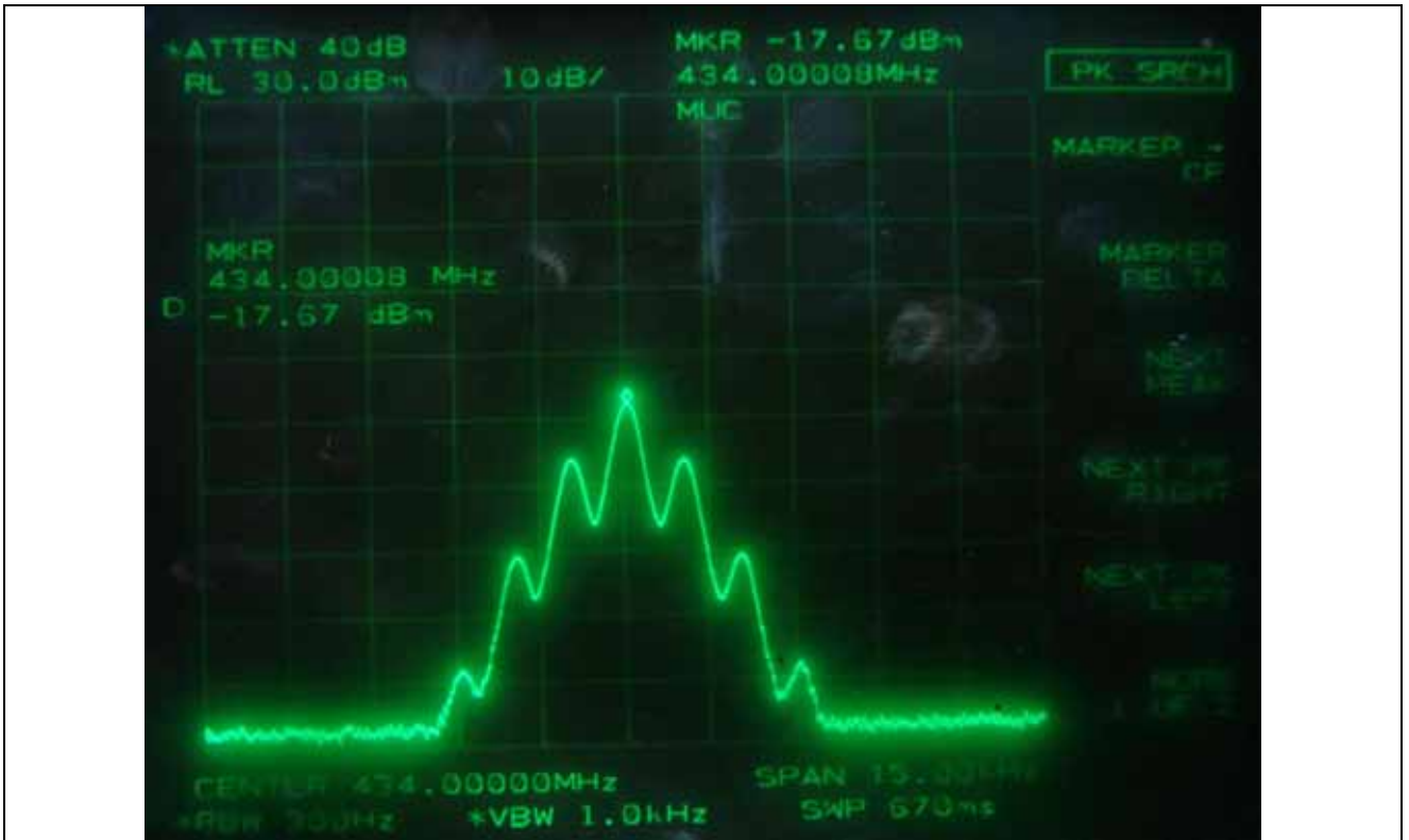
FM with 2.5 kHz sine wave signal, Channel Spacing 6.25 kHz - Input (High Channel)
