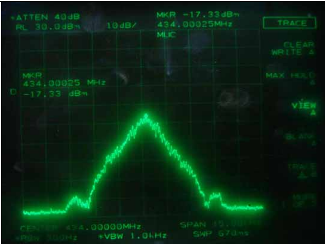
FM with an external 9 600 b/s random data source, Channel Spacing 6.25 kHz - Input (Low Channel)
