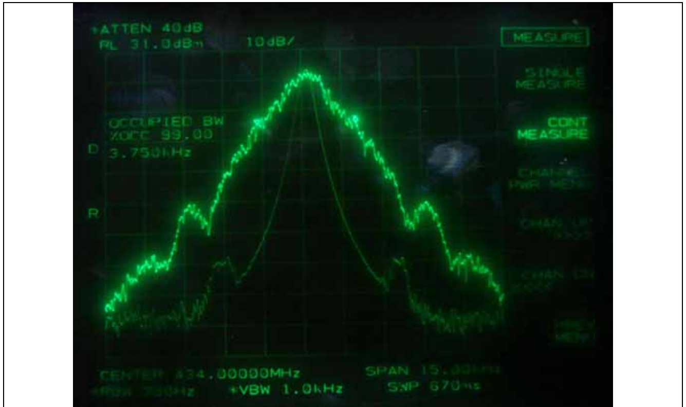
FM with an external 9 600 b/s random data source, Channel Spacing 6.25 kHz - High Channel
