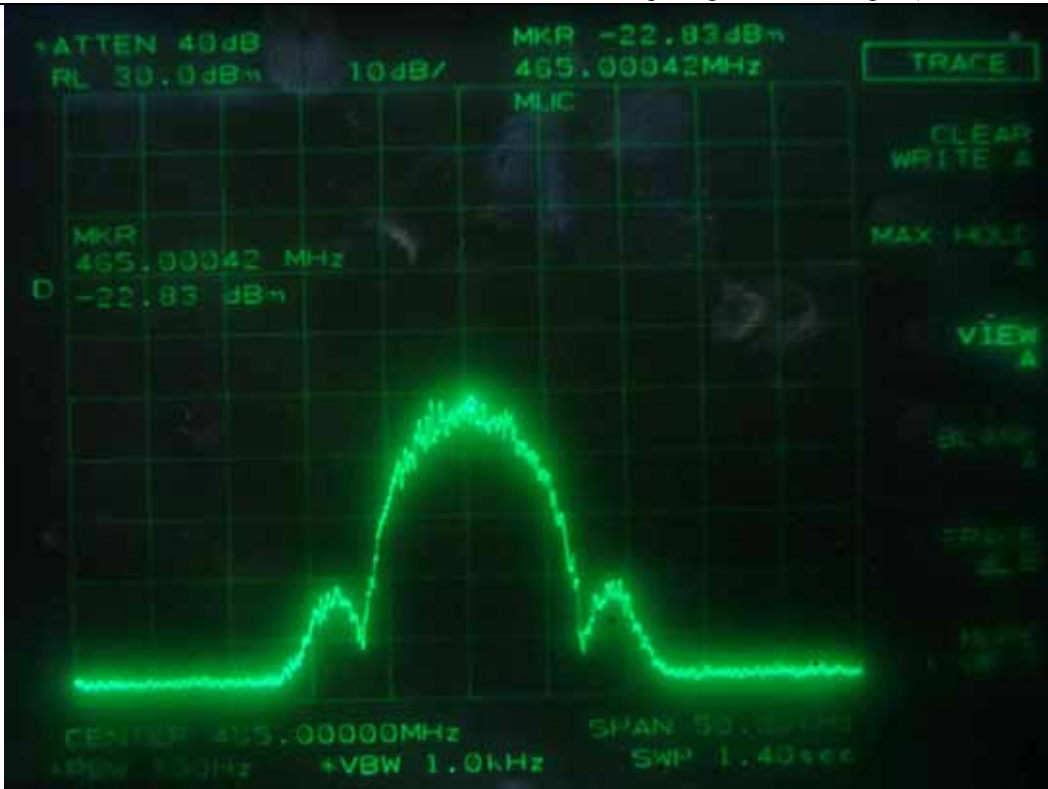
FM with an external 9 600 b/s random data source, Channel Spacing 12.5 kHz - Input (Middle Channel)
