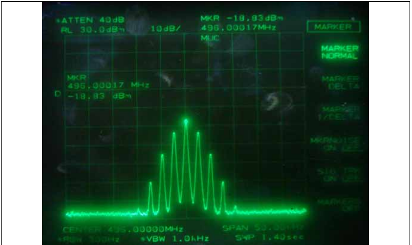
FM with 2.5 kHz sine wave signal, Channel Spacing 12.5 kHz - Input (High Channel)
