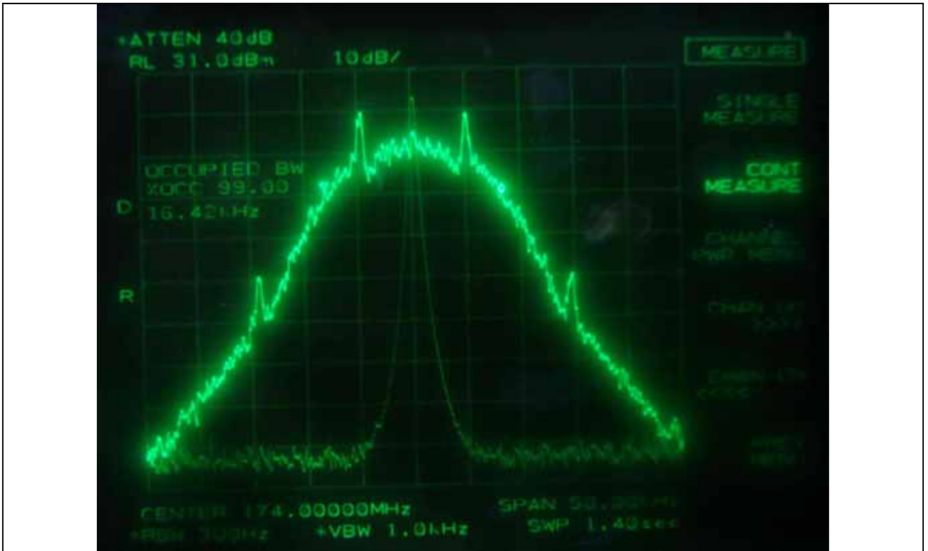
FM with an external 9 600 b/s random data source, Channel Spacing 25 kHz - High Channel
