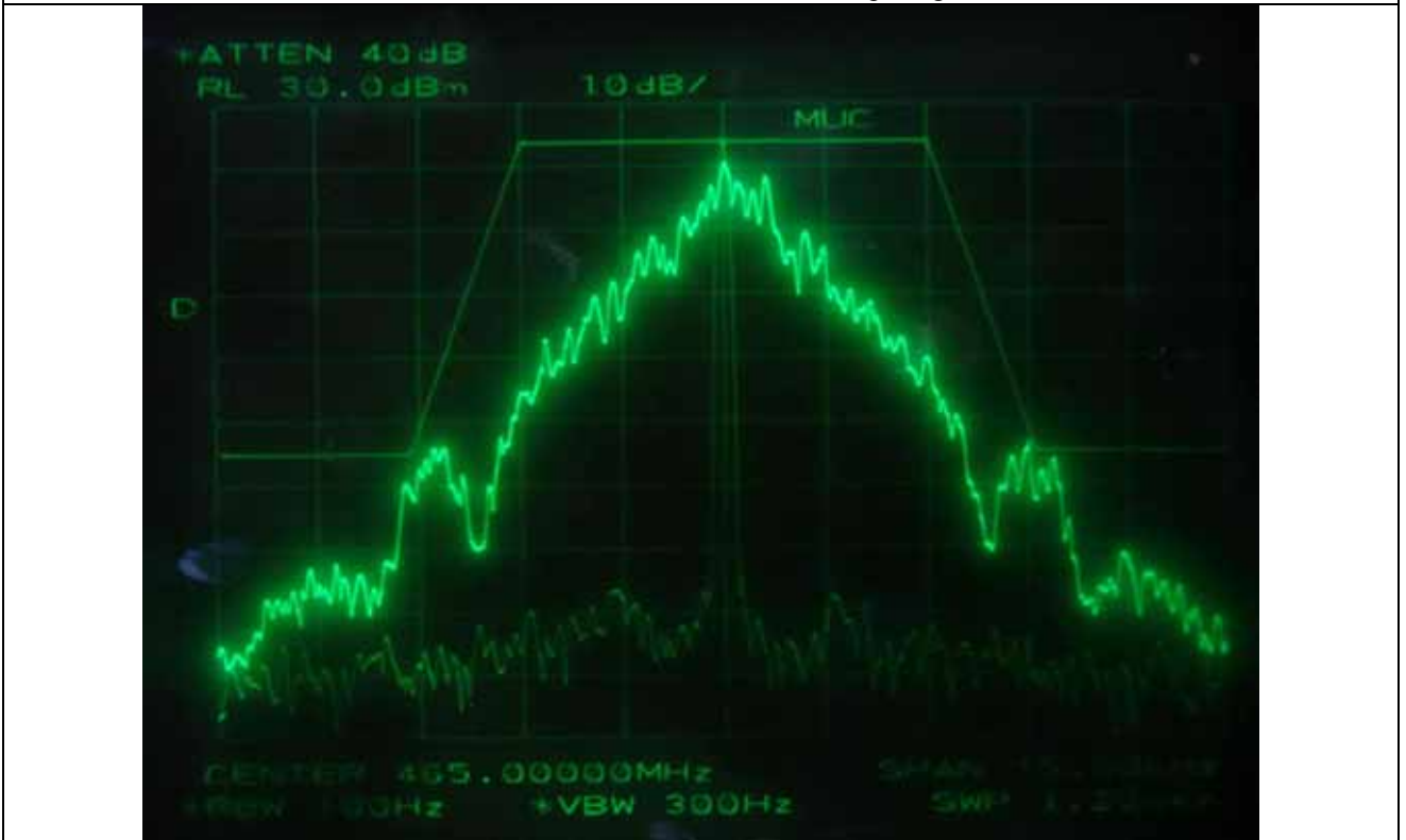
FM with an external 9 600 b/s random data source, Channel Spacing 6.25 kHz - Middle Channel
