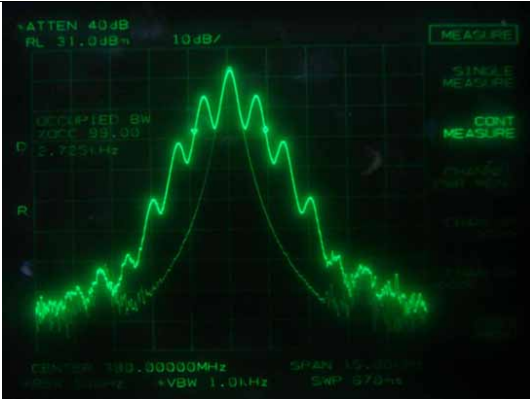
FM with 2.5 kHz sine wave signal, Channel Spacing 6.25 kHz - Low Channel
