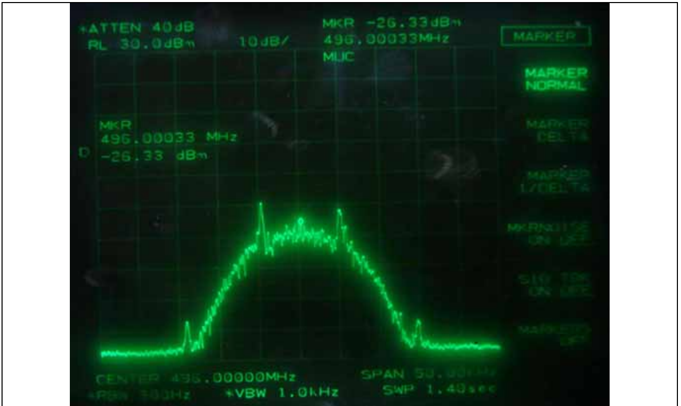
FM with an external 9 600 b/s random data source, Channel Spacing 25 kHz - Input (High Channel)
