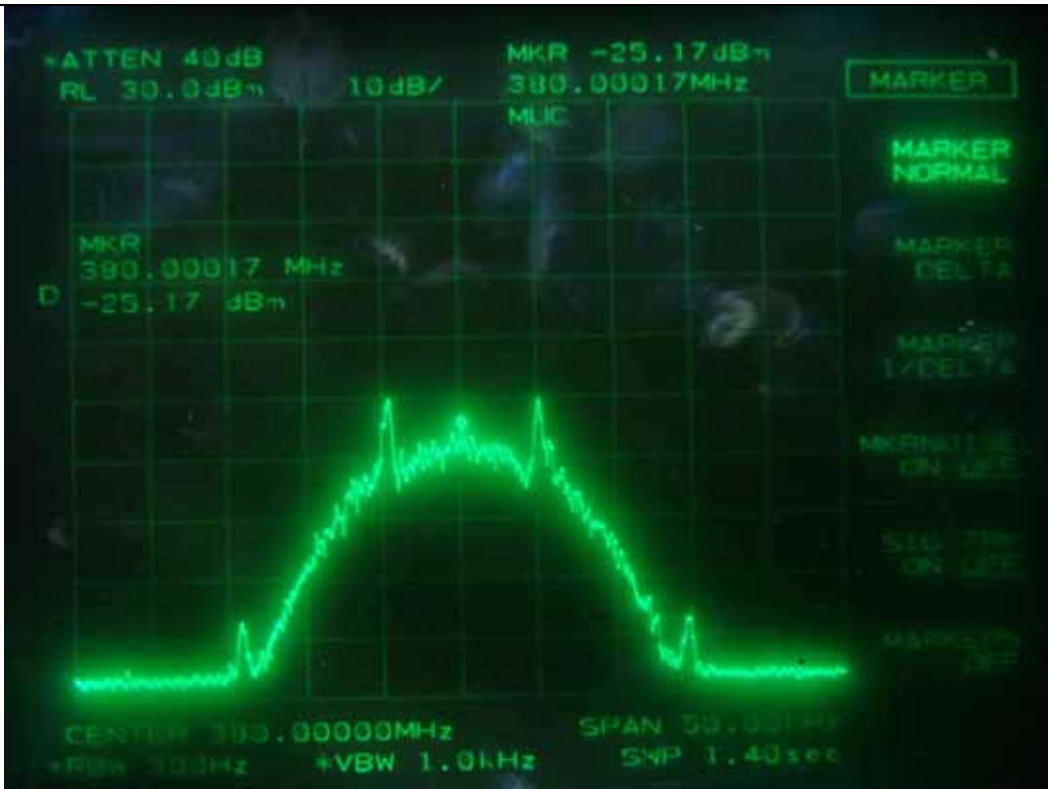
FM with an external 9 600 b/s random data source, Channel Spacing 25 kHz - Input (Low Channel)
