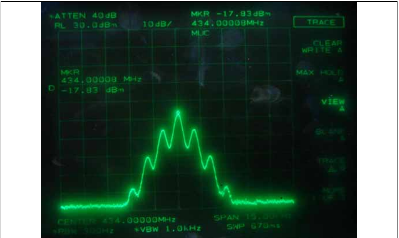
FM with 2.5 kHz sine wave signal, Channel Spacing 6.25 kHz - Input (Low Channel)
