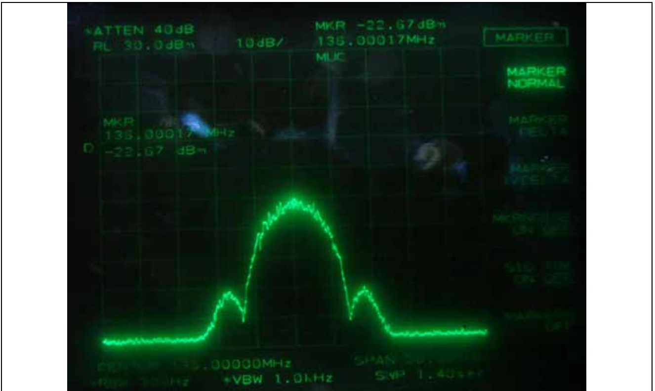
FM with an external 9 600 b/s random data source, Channel Spacing 12.5 kHz - Input (Low Channel)
