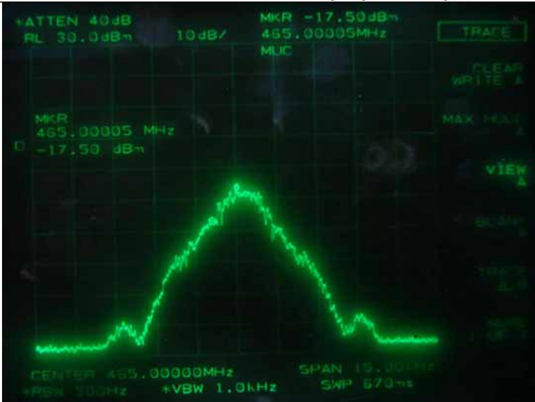
FM with an external 9 600 b/s random data source, Channel Spacing 6.25 kHz - Input (Middle Channel)
