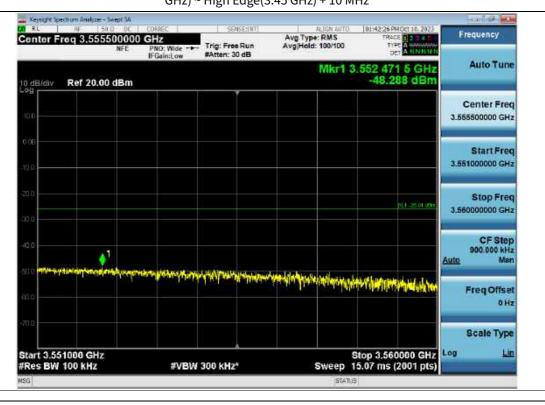
Spurious / 3.7 GHz Service(High) + 3.45 GHz Service(Low) (ANT 2) / Downlink / 5G NR 20 MHz / High Edge(3.45
