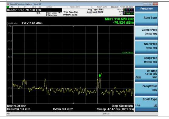
Spurious / 3.7 GHz Service(High) + 3.45 GHz Service(Low) (ANT 2) / Downlink / 5G NR 20 MHz / 9 kHz ~ 150 kHz
