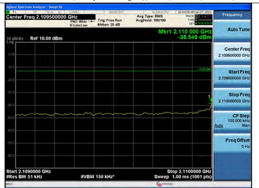
+3 dB above Out-of-band (two adjacent test signals) / AWS13 / Downlink / LTE 5 MHz / Lower
