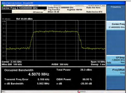
3 dB above the AGC threshold output / AWS13 / Downlink / LTE 5 MHz
