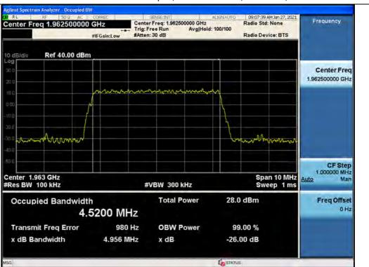
3 dB above the AGC threshold output / Broadband PCS / Downlink / LTE 5 MHz
