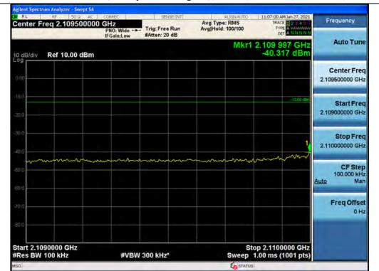
+3 dB above Out-of-band (two adjacent test signals) / AWS13 / Downlink / LTE 10 MHz / Lower
