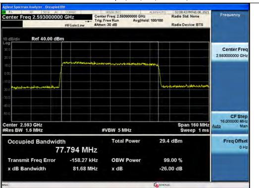
3 dB above the AGC threshold output / BRS/EBS / Downlink / 5G NR 80 MHz
