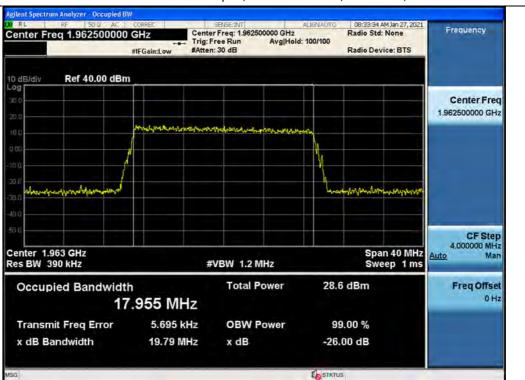
3 dB above the AGC threshold output / Broadband PCS / Downlink / LTE 20 MHz
