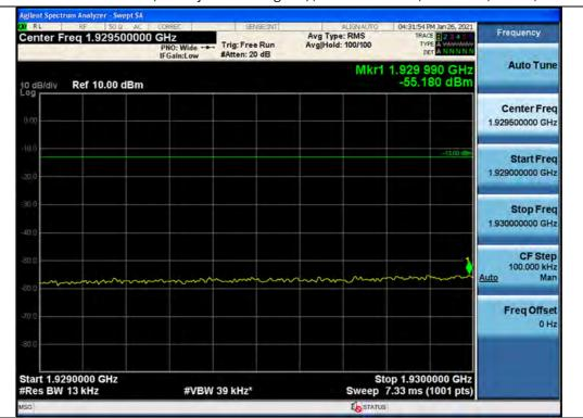
+3 dB above Out-of-band (two adjacent test signals) / Broadband PCS / Downlink / CDMA / Lower
