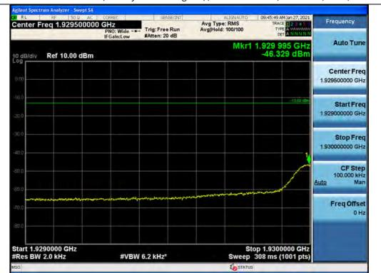
+3 dB above Out-of-band (two adjacent test signals) / Broadband PCS / Downlink / GSM / Lower
