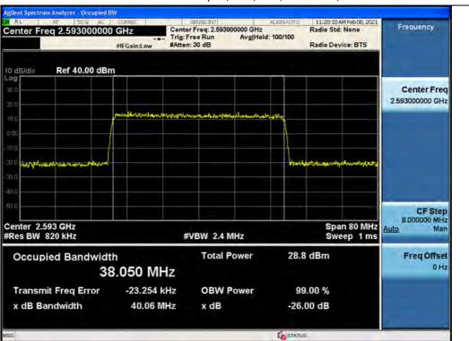
3 dB above the AGC threshold output / BRS/EBS / Downlink / 5G NR 40 MHz
