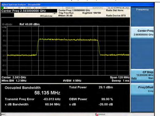
3 dB above the AGC threshold output / BRS/EBS / Downlink / 5G NR 60 MHz
