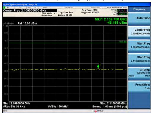
+3 dB above Out-of-band (two adjacent test signals) / AWS13 / Downlink / WCDMA / Lower
