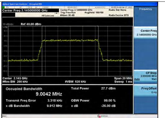
3 dB above the AGC threshold output / AWS13 / Downlink / LTE 10 MHz
