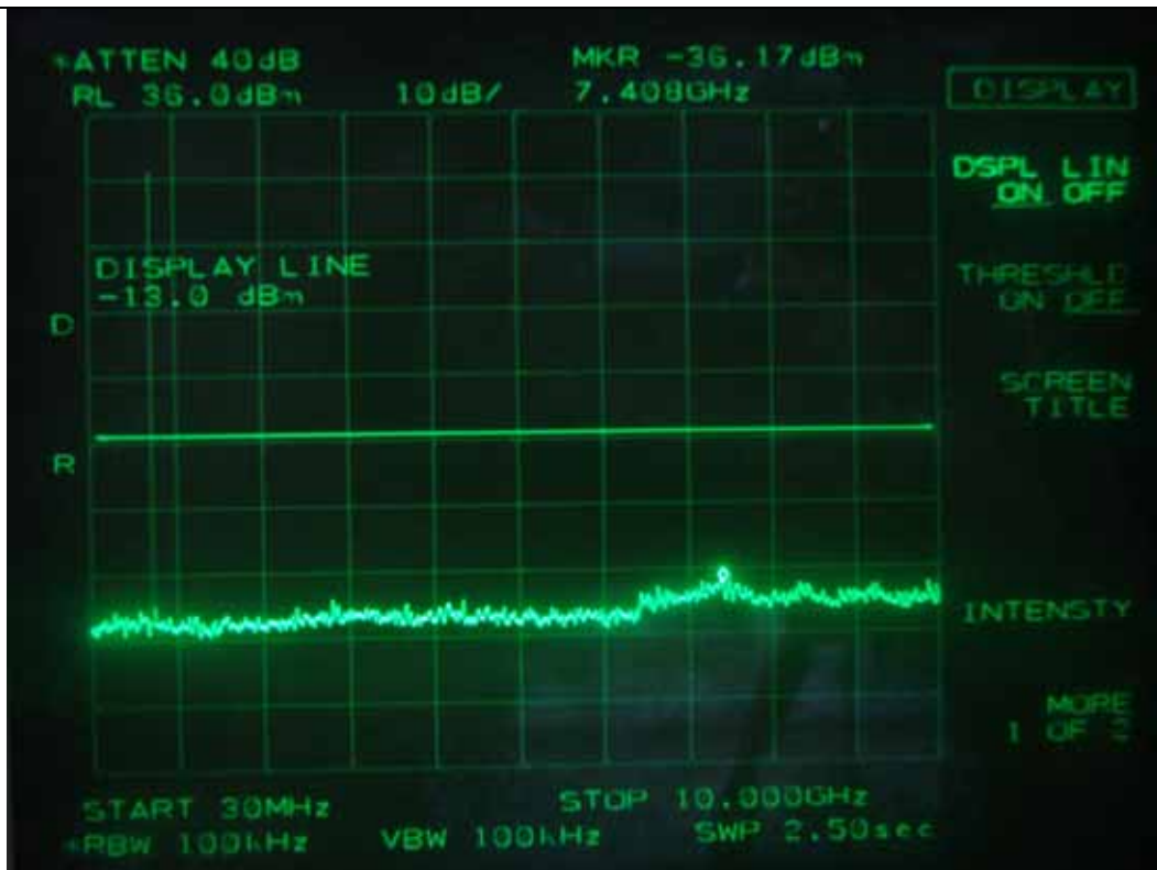
Low Channel – 3 input signals
