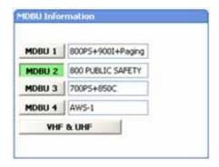
Check if MDBU is inserted into a corresponding slot of BIU. The ID screen shows the following:
