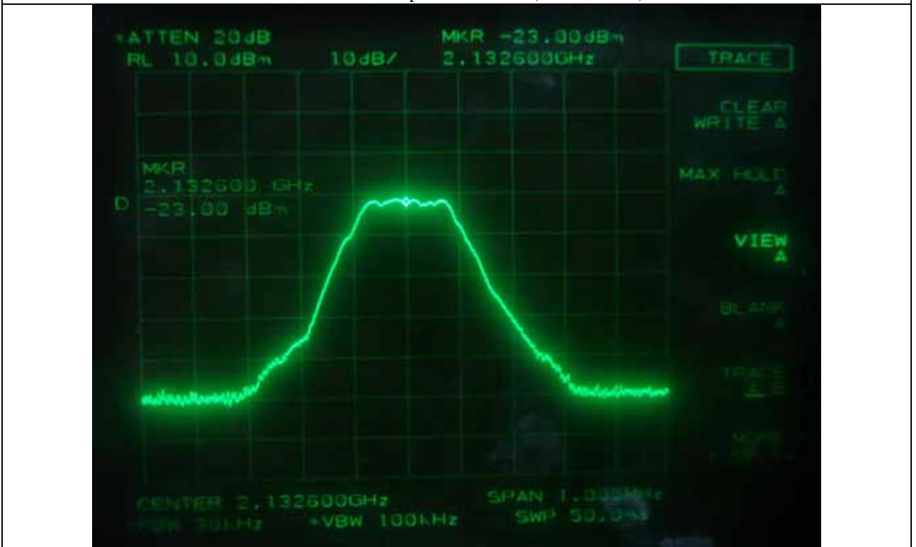
GSM – 99 % Occupied Bandwidth (Middle Channel)
