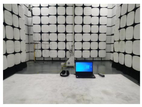
1.2.Photos of Radiated Emission Test (In Semi Anechoic Chamber above 1GHz)
