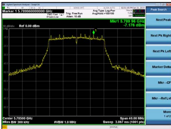
(802.11a) PSD plot on channel 165
