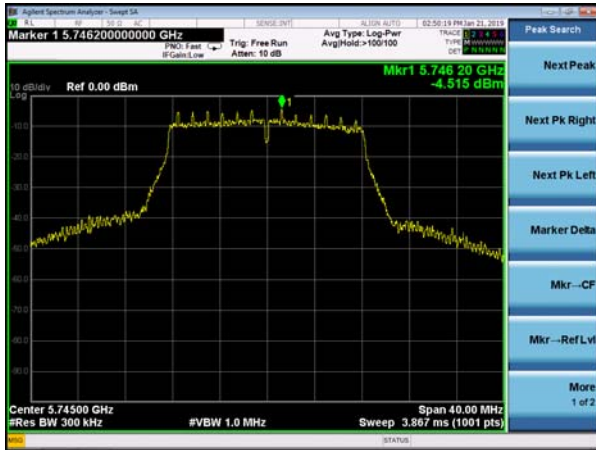
(802.11a) PSD plot on channel 157
