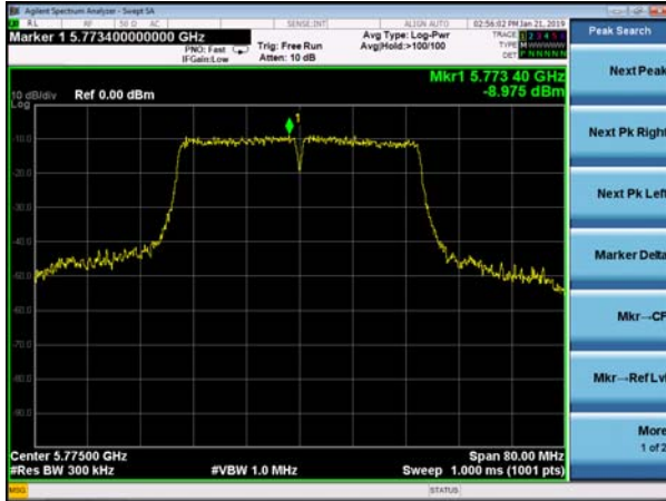
(802.11n40) PSD plot on channel 159
