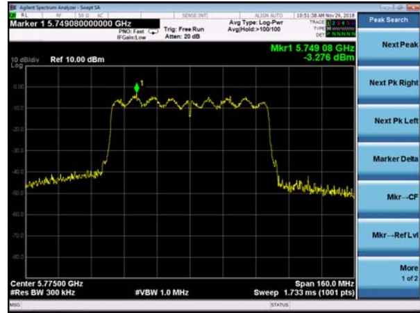
(802.11ac80) PSD plot on channel 155
