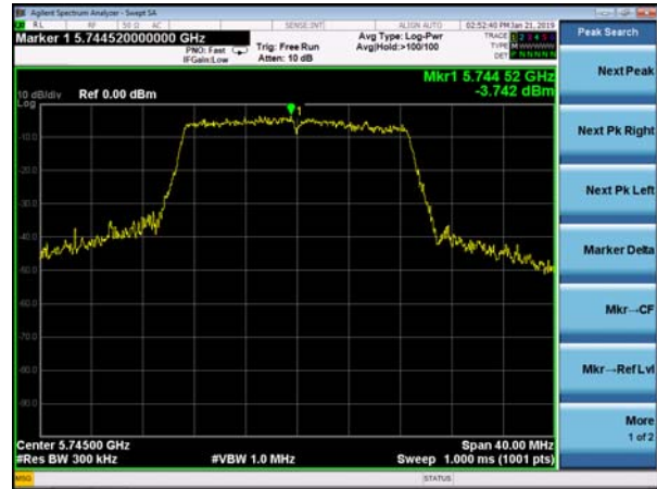
(802.11n20) PSD plot on channel 157
