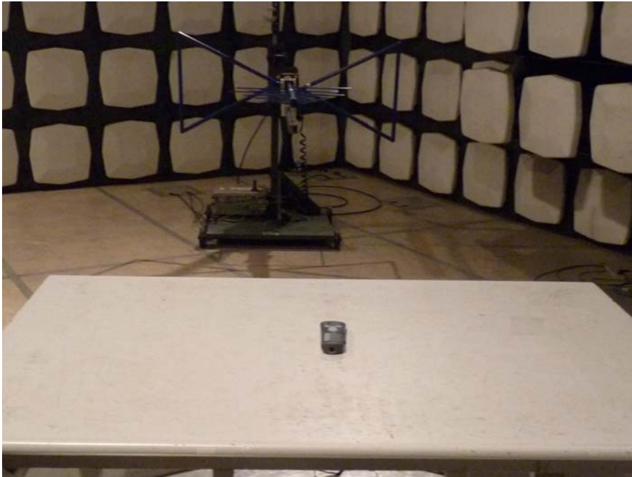
Figure 1 Test photo of Transmitter Spurious Emission (TX Mode 30-1000MHz)
