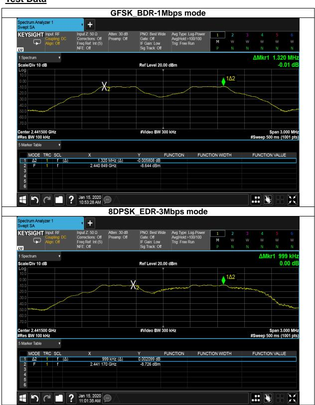
Note: We selected worst case to performed test in middle channel, The results can be meet other channel.
