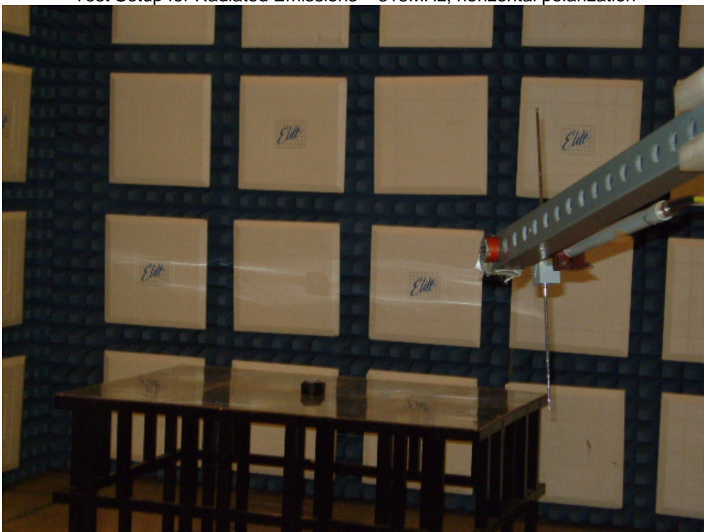
Test Setup for Radiated Emissions – 315MHz, vertical polarization
