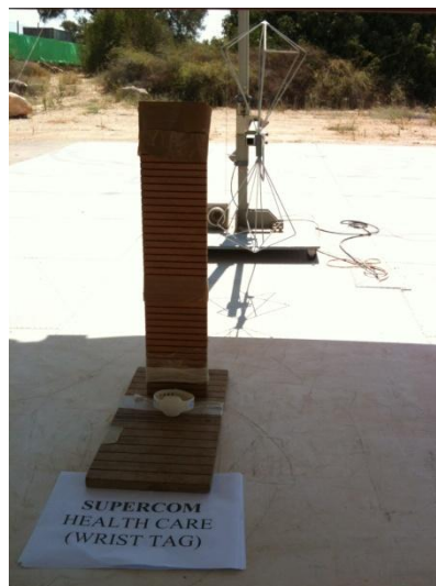
Figure 7. Radiated Emission Test – Wrist Tag PRF-HCT20WT
