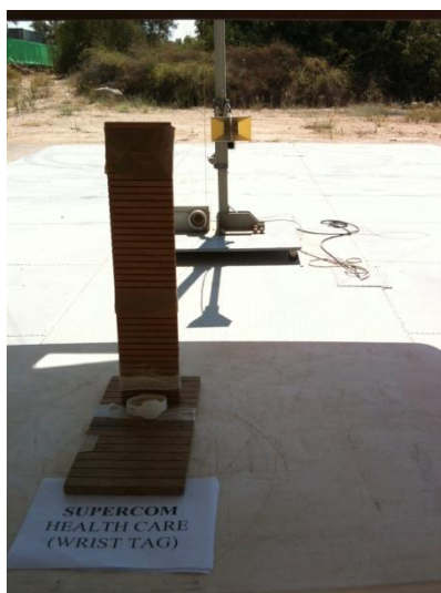
Figure 9. Radiated Emission Test – Wrist Tag PRF-HCT20WT
