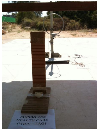
Figure 6. Radiated Emission Test – Wrist Tag PRF-HCT20WT
