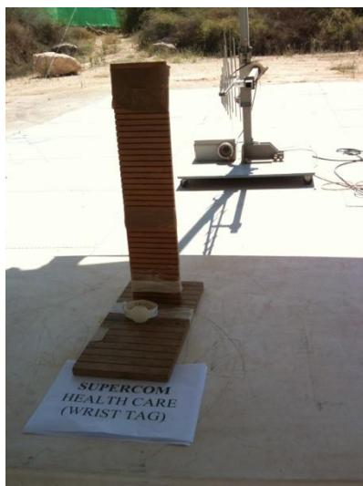
Figure 8. Radiated Emission Test – Wrist Tag PRF-HCT20WT
