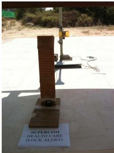
Figure 5. Radiated Emission Test - Lock Alert PRF-HCT20LA
