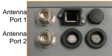
Figure 38 – Antenna ports of LPR® Station
