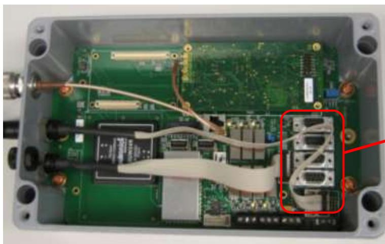
Figure 25 Internal view of LPR® Station
