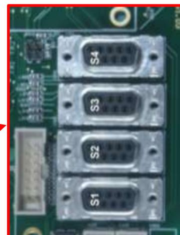
Figure 26 – Internal Data Interfaces
