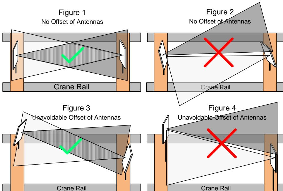
Figure 19 Antenna Position with and without Offset
