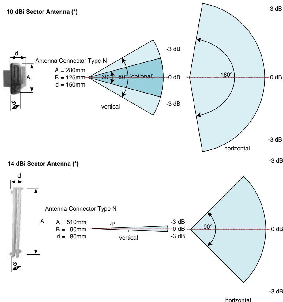
*Figure 15: Example of directional characteristic of typical LPR® antennas*
