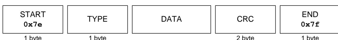
Figure 1: Structure of data the packet
