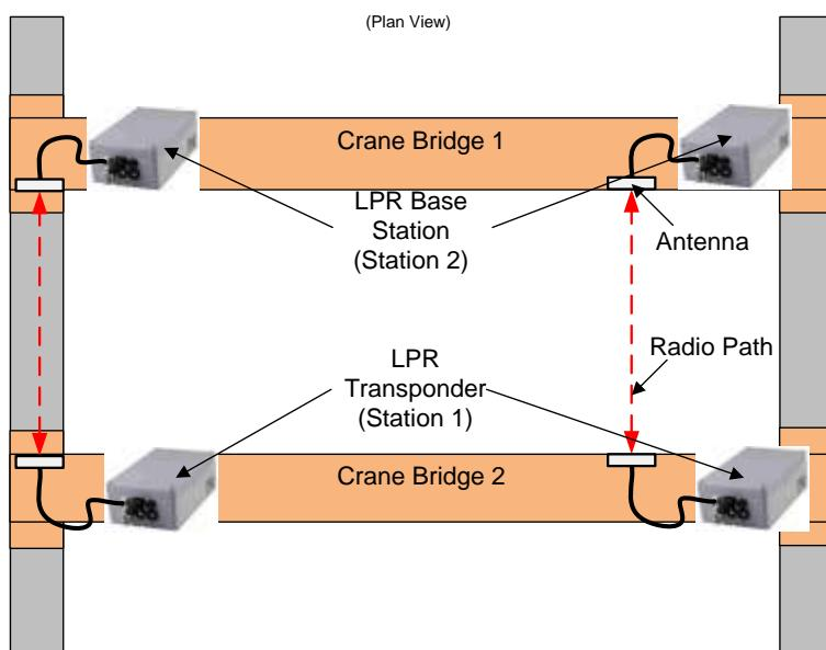
Figure 6: LPR® 1DX Redundant arrangement
