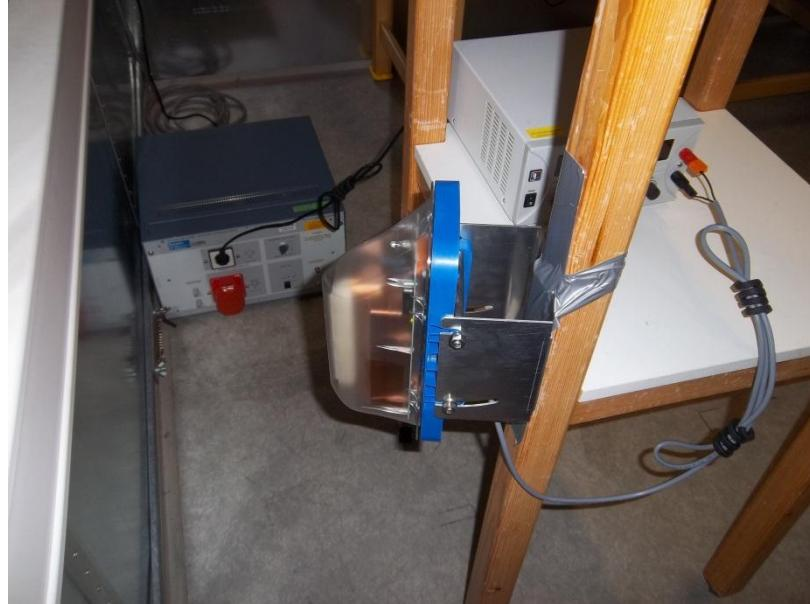
radiated disturbance 9kHz – 30MHz
