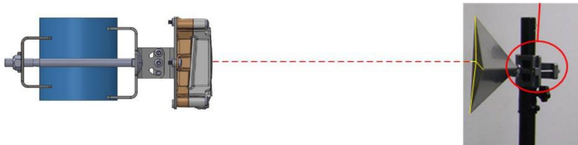
Figure 5.1: Mounting alignment of radar and reflector
