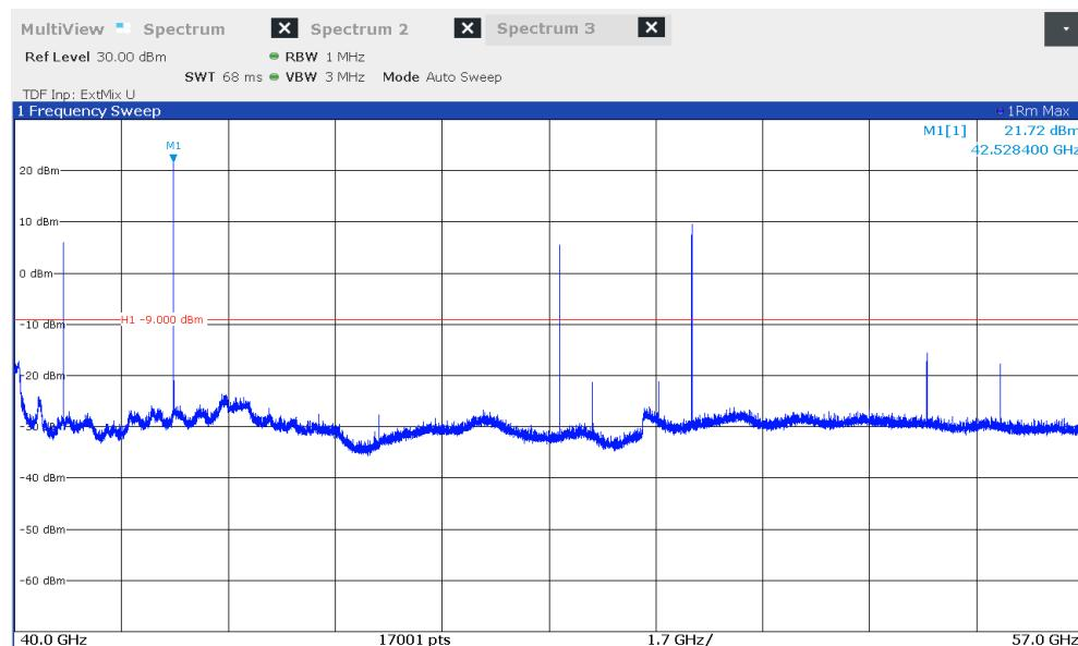
Note: The emission 40.906 GHz, 42.528 GHz, 48.871 and 50.996 GHz are caused by the external Mixer.
