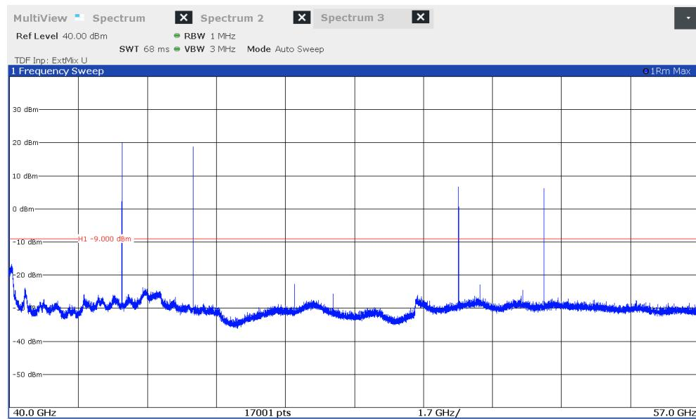
Note: The emission 42.722 GHz, 44.515 GHz, 50.957 and 53.082 GHz are caused by the external Mixer.
