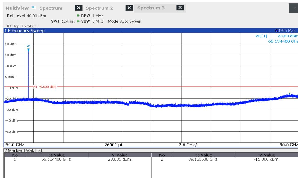
Note: The emission 66.134 GHz is caused by the external Mixer.
