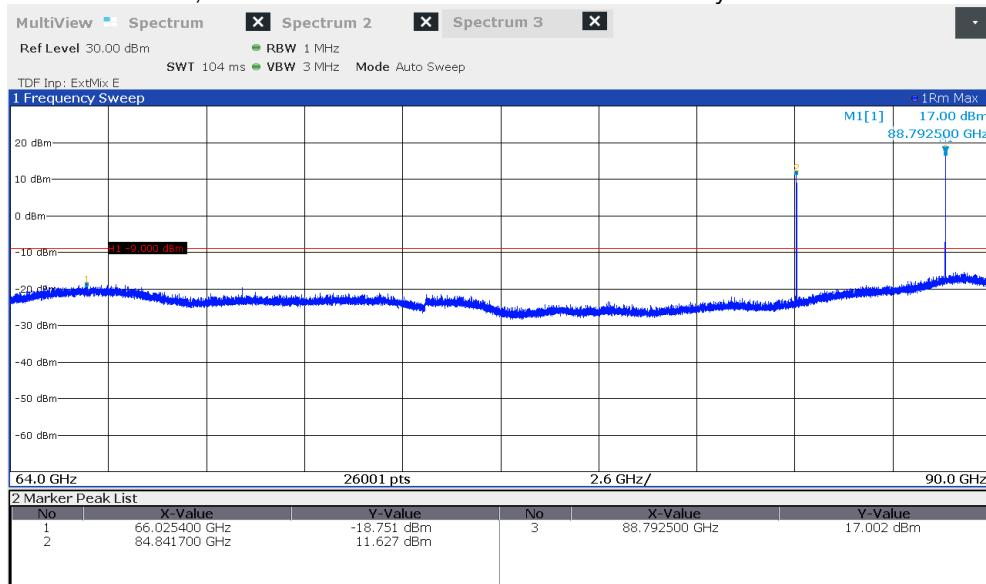
Note: The emission 84.841 GHz and 88.792 GHz are caused by the external Mixer.
