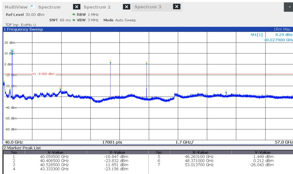
Note: The emission 40.528 GHz, 46.263 GHz and 48.371 GHz are caused by the external Mixer.
