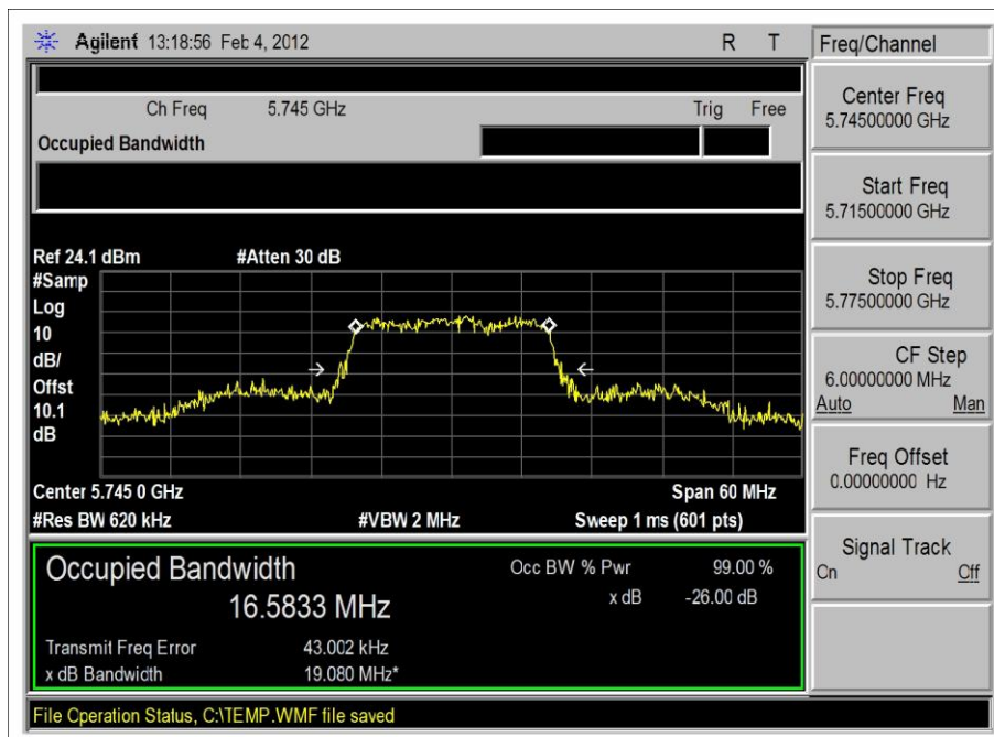
802.11a - Antenna Port 1
